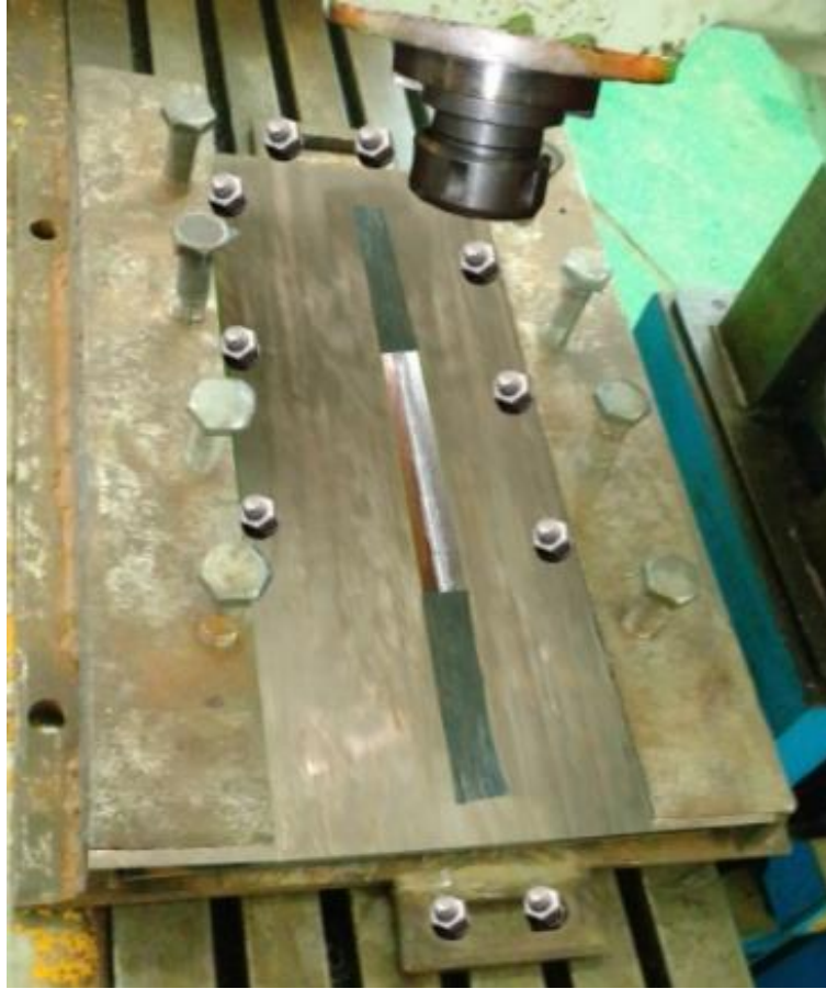
Figure 3-1 FSW setup on CVMM
