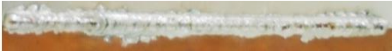
f) 1600 rpm, 20mm/min and 1mm (weld 6)
