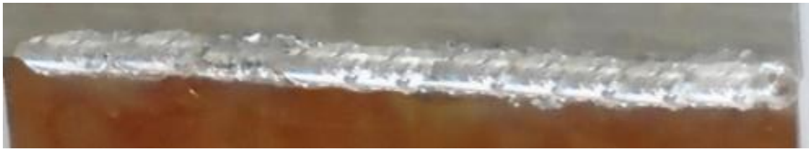
a) 1000 rpm, 12.5mm/min and 1mm (weld 1)
