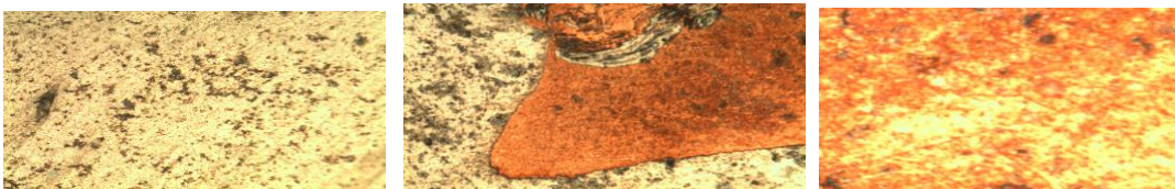
c) Microstructure at 1000 rpm, 20mm/min and 2mm (weld 3)
