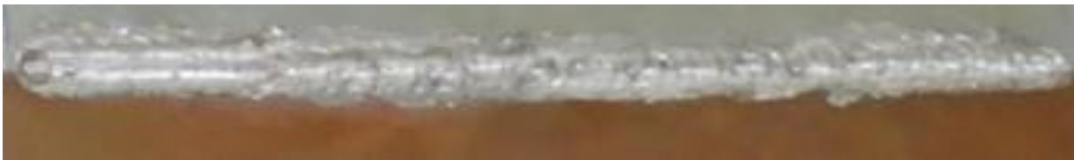
b) 1000 rpm, 16mm/min and 1.5mm (weld 2)
