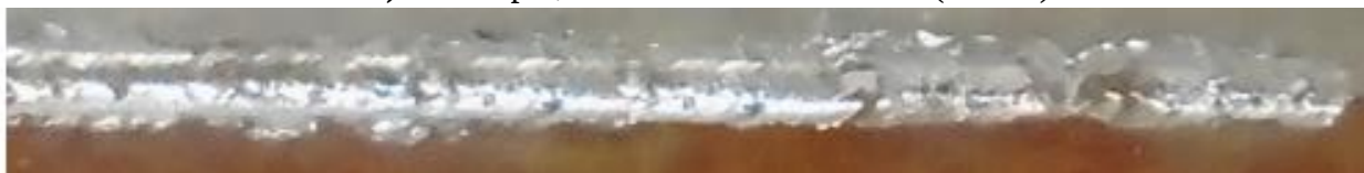
d) 1250 rpm, 12.5mm/min and 1.5mm (weld 4)
