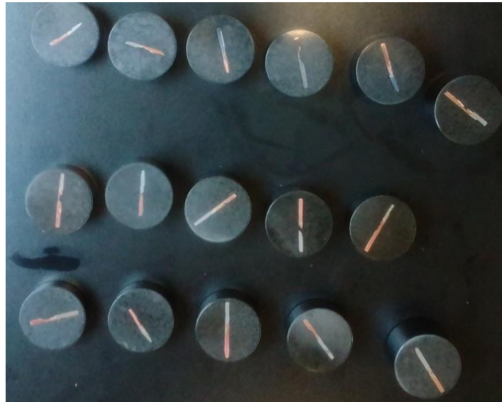
Figure 4-6 Mounted FSW joints for Micro-structure and hardness
