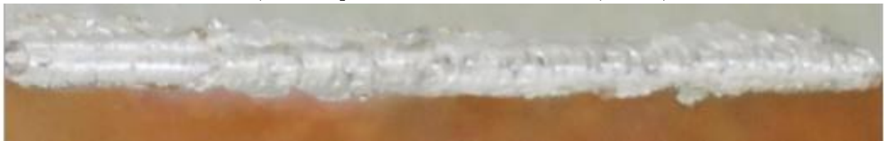
b) 1000 rpm, 16mm/min and 1.5mm (weld 2)
