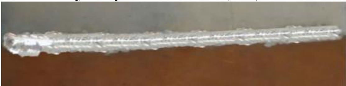
h) 1600 rpm, 16mm/min and 1mm (weld 8)
