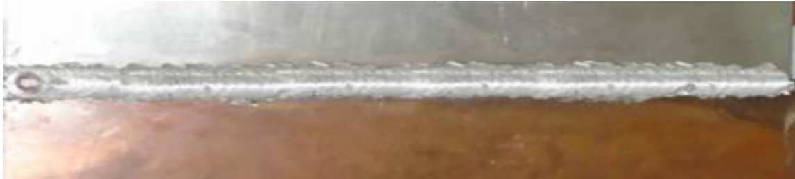
g) 1600 rpm, 12.5mm/min and 2mm (weld 7)
