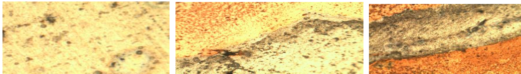
e) Microstructure at 1250 rpm, 16mm/min and 2mm (weld 5)
