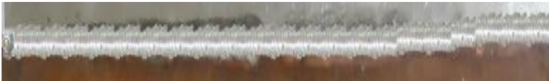
h) 1600 rpm, 16mm/min and 1mm (weld 8)
