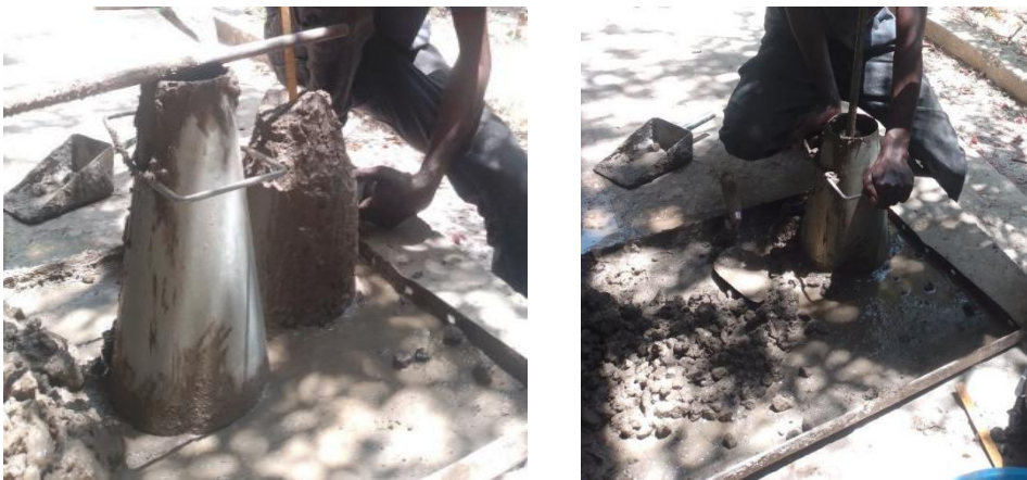
Figure 3. 6 : Slump test process
