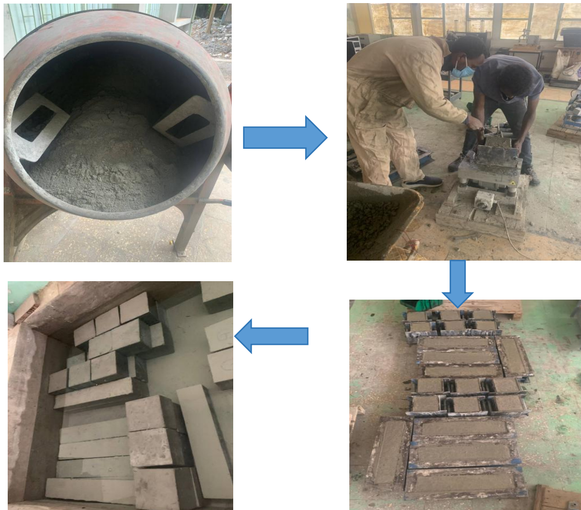
Figure 3. 5 Process of mixing sample,vibrating and curing
