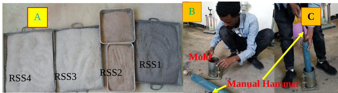
Figure 3. 13 : Compacted test of soil from critical slope section of my study area, A) Soil sample preparation for compaction B) Fixing the molds.
