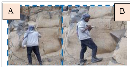
Figure 3. 1: In-situ strength test using Schmidt hammer A) Smoothing the rock and make square B) Taking the rebound value (R)
