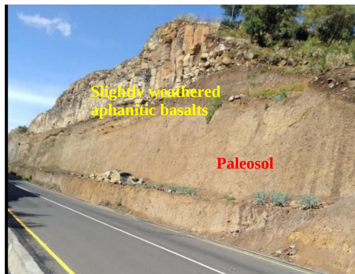
Figure 4. 11. Aphanitic basalts underline by paleosol
