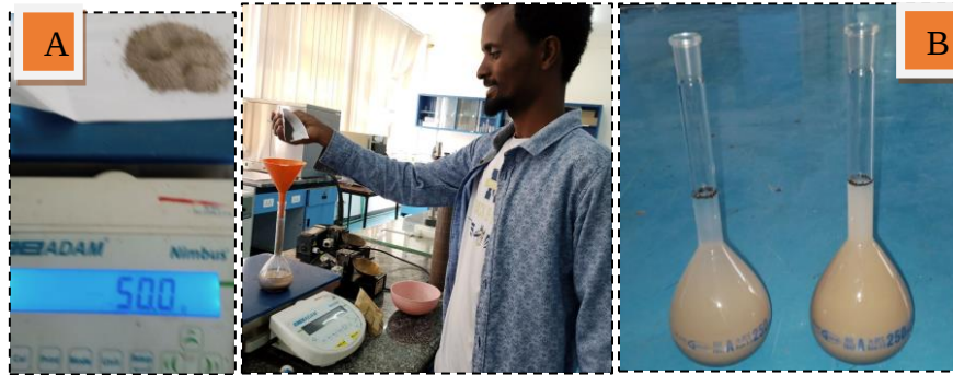
Figure 3. 12: specific gravity for soils A) Soil sample with digital balance B) Pycnometer filled with water and soil
