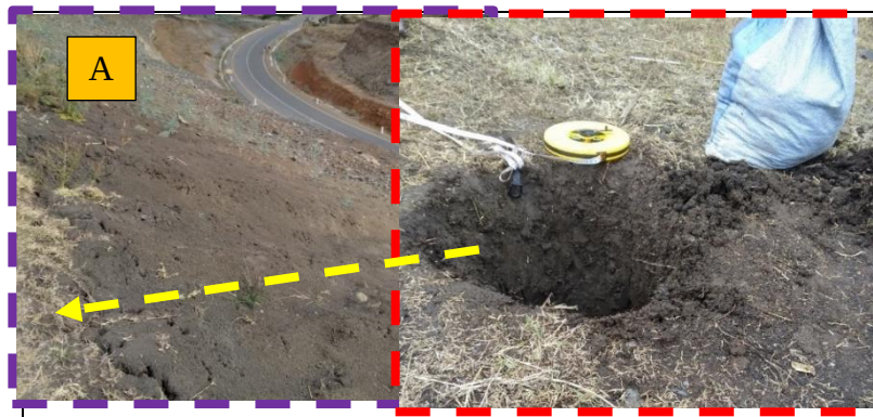
Figure 3. 3: Critical soil slope section and its sample (black cotton soil, SS1)
