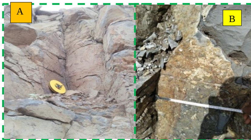
Figure 4. 9. A) Moderately weathered aphanitic basalt of columnar joint B) slightly weathered aphanitic basalt
