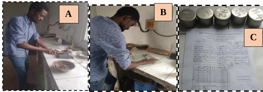
Figure 3. 11: Atterberg limit test for soils A) Liquid limit (LL) B) Plastic limit (PL) C) Moisture cans for both LL and PL
