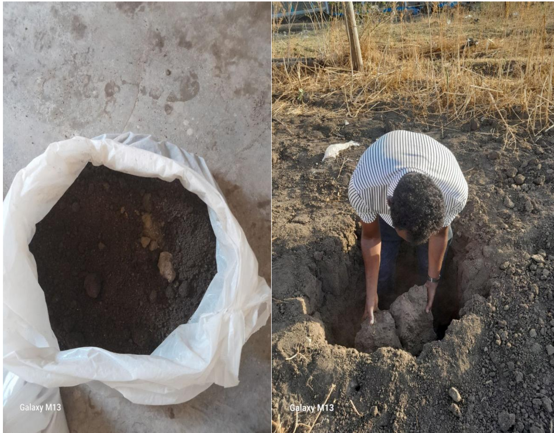
Figure 3. 2: Expansive soil sample and during sampling from pit at digging stage
