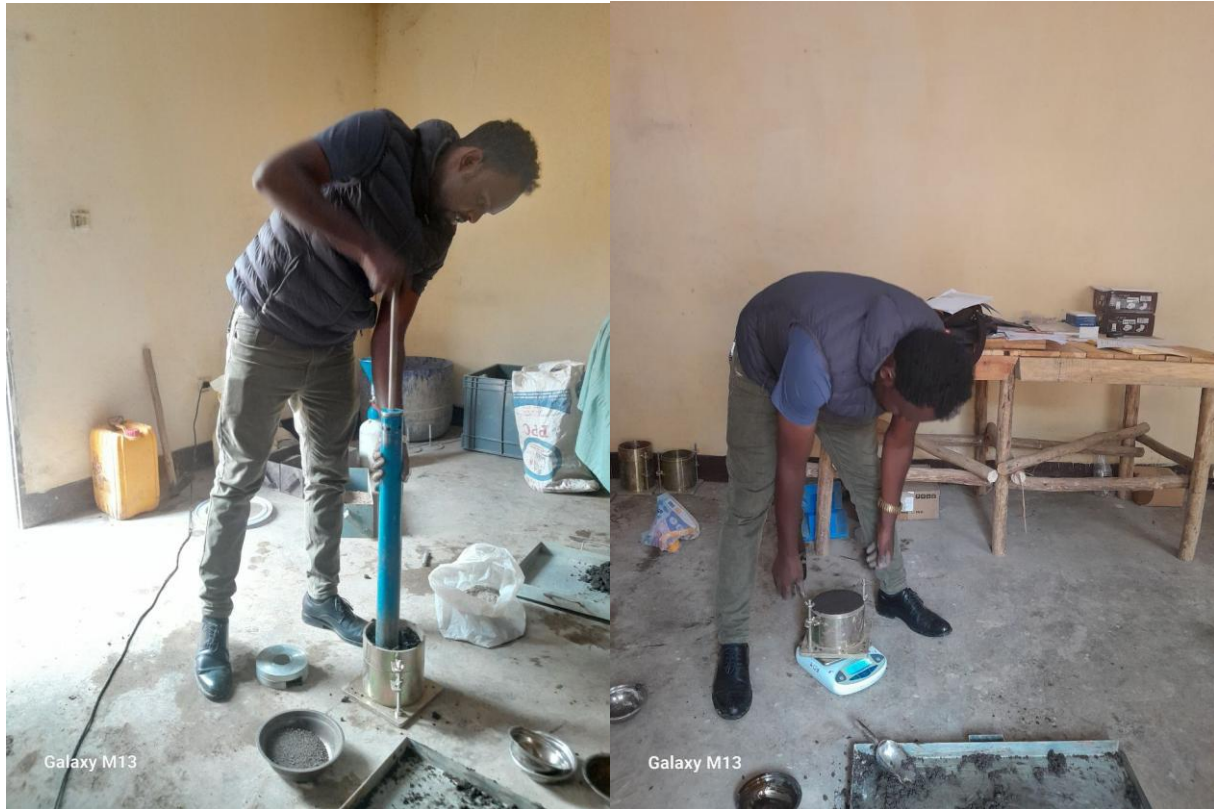
Figure 3. 4: compaction test apparatus and while conducting the test
