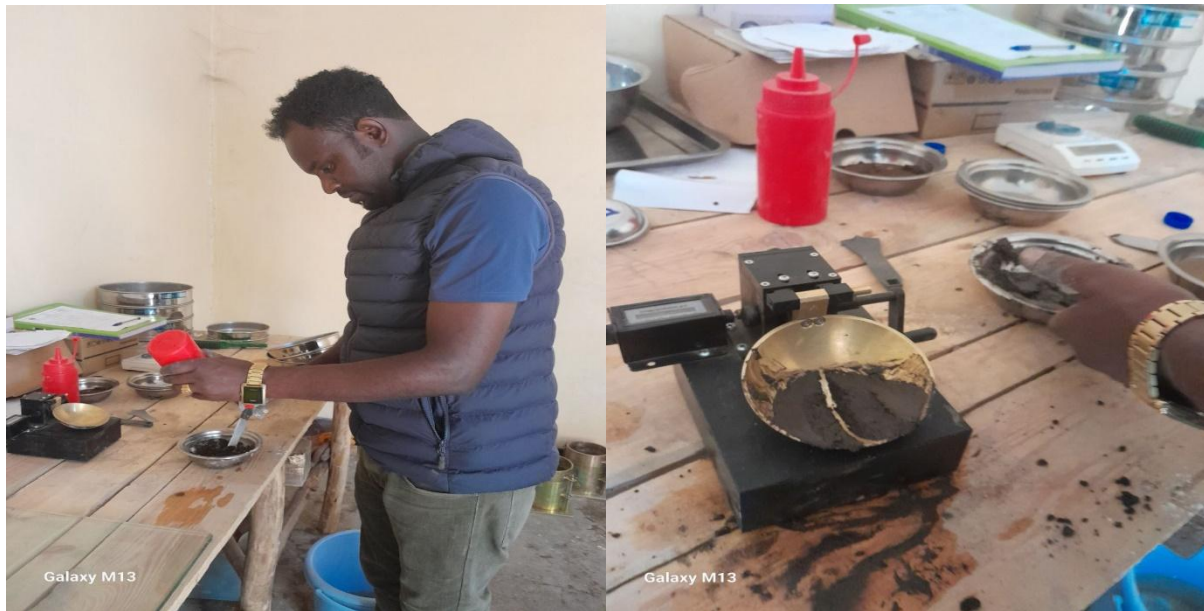
Figure 3.3: while testing liquid limit test and apparatus used.
