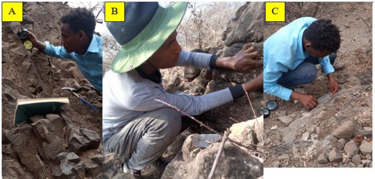
Figure 3. 1 Discontinuity survey from abutments and reservoir: A) Measuring dip direction and dip amount using Brunton compass, B & C Measuring discontinuity characteristics using ruler.
