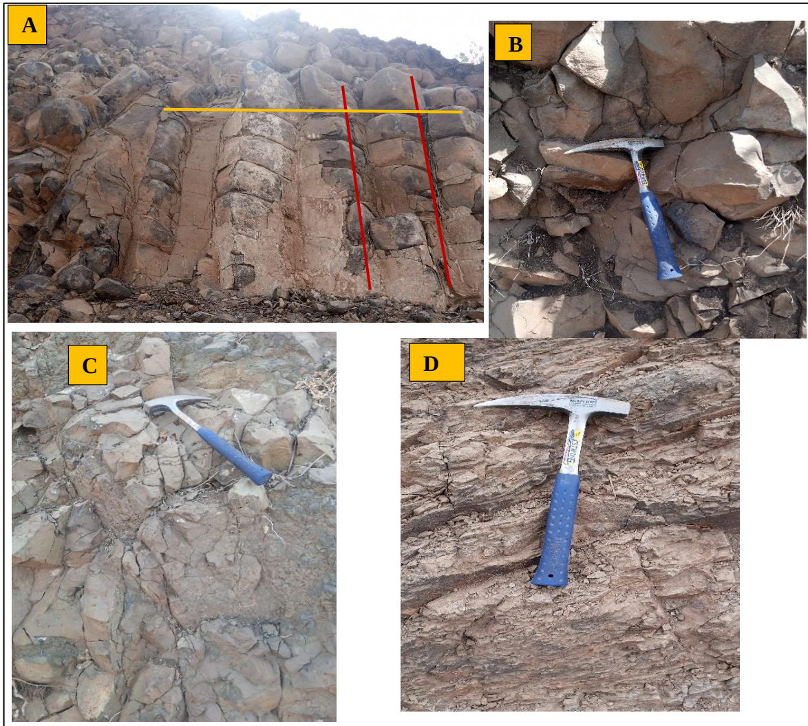
Figure 4. 4 Different joints at (A) Spill way, (B & C) right abutment and (D) left reservoir rim
