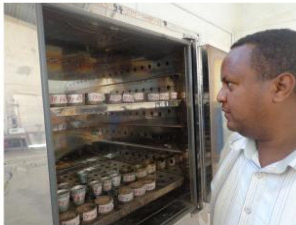
Fig. C.6 Test Samples under Oven Dry Condition
