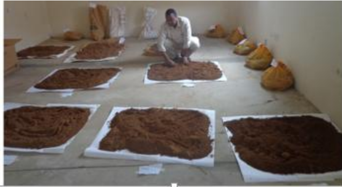
Fig. C.5 Test Samples under Air Drying Condition
