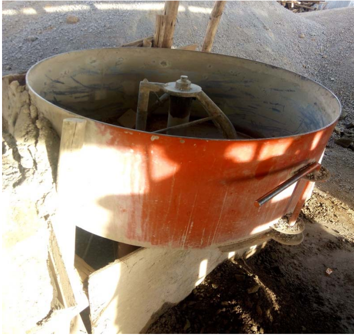
Fig.5.7. Mixer for HCB production at Atana Tera
