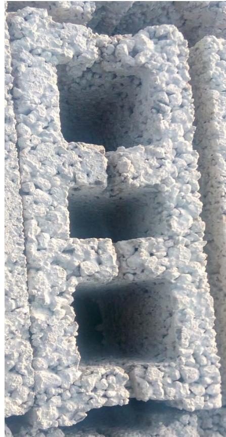
Fig. 5.12. HCB of three holes and good texture Fig. 5.13. HCB of three holes and poor texture
