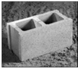
Fig 3.1. Hollow concrete block
