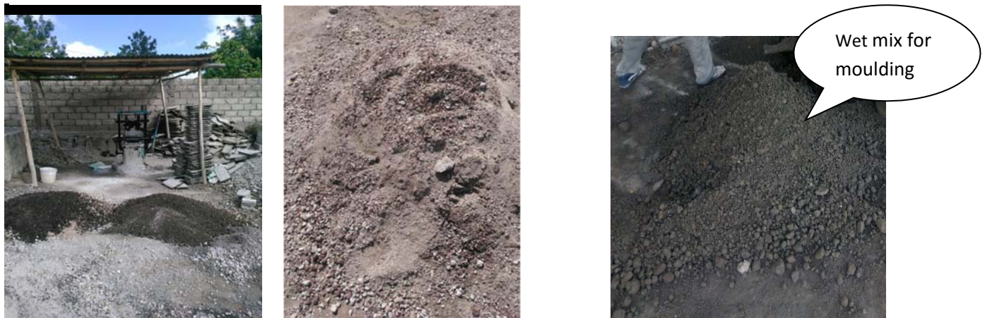
Fig. 5.6. Hand mixing and proportioning
