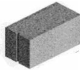
Fig. 3.2. solid concrete block
