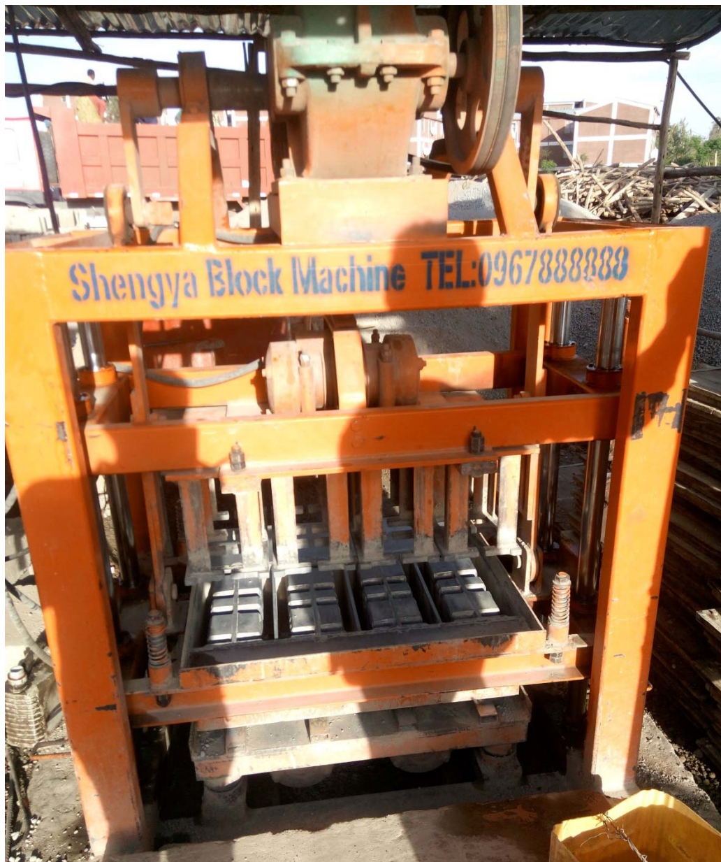
5.8. Automated HCB producing machine around Atanatera (res. 17)
