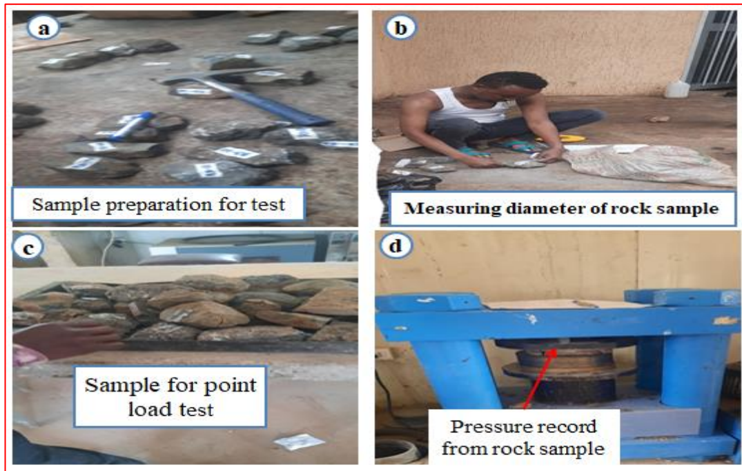
Figure4.9: point load strength test of intact rocks
