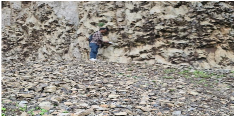
Figure 4.2: In-situ strength rock test using Schmidt hammer rebound value for the estimation of uniaxial compressive strength (UCS).
