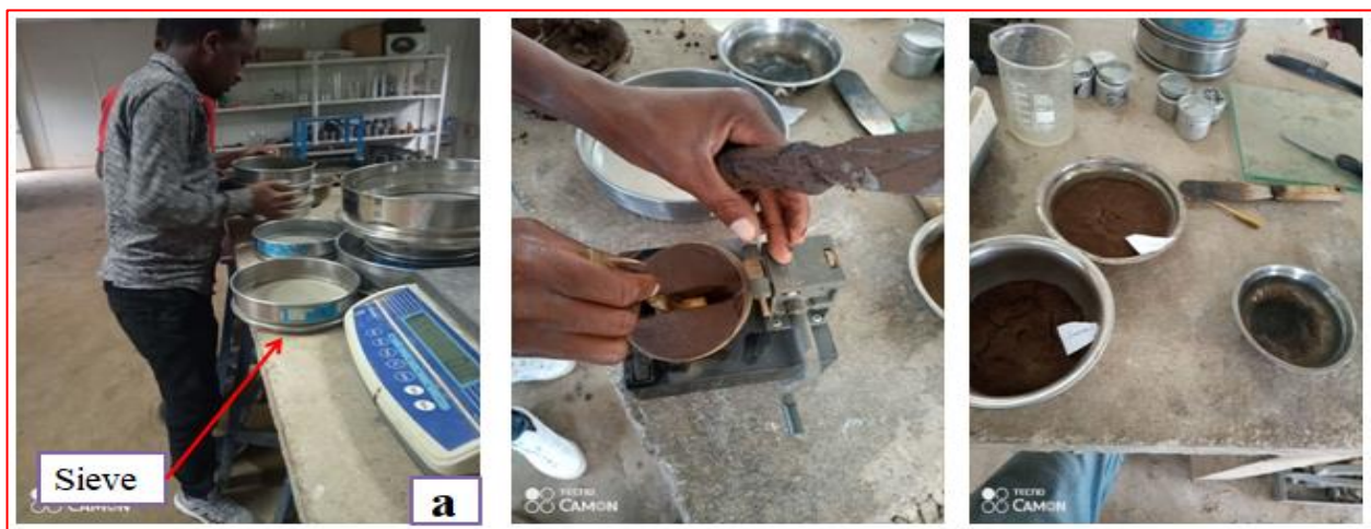
Figure4.5: Sieve and Atterberg limit tests of soils
