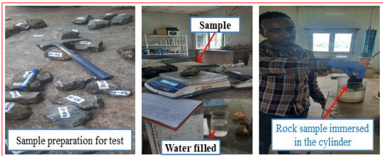
Figure4.10: Unit weight testing of rock samples
