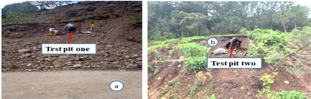
Figure4.3: Pits for soil sampling at a) SS1 and b) SS2
