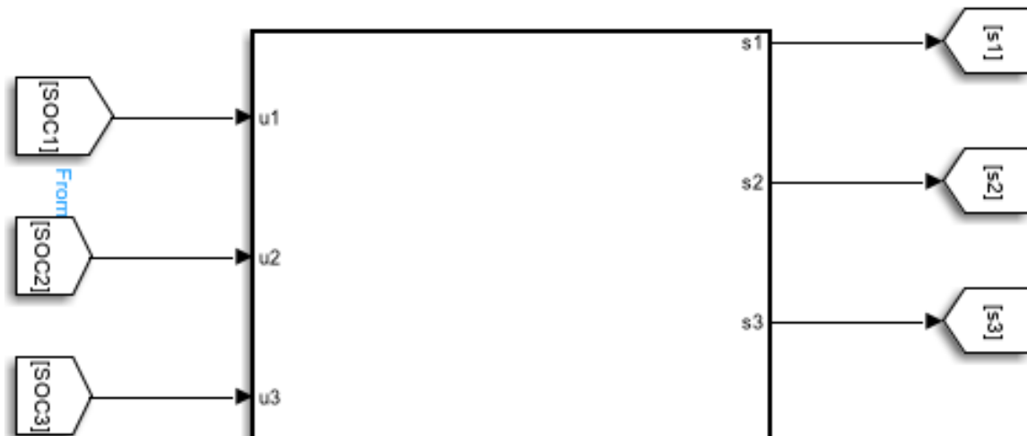
Figure 3.13: MATLAB function block connecting SOC monitor to Ideal switch
