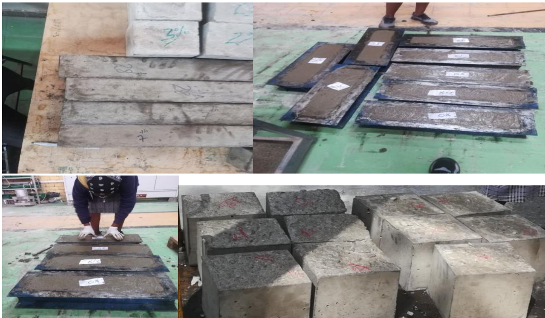
Appendix C 2 : Pictures shows casted samples: sized cube for compressive, beam, water absorption test and Sulfate attack test.
