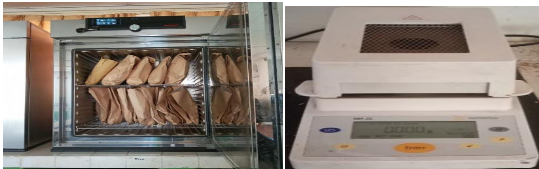
Figure 10: Oven and moisture analyzer used for analysis
