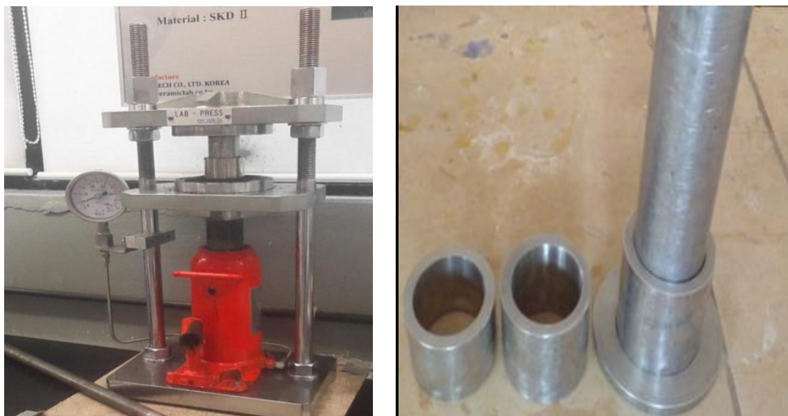
Figure 12: Mechanical press and cylindrical die for briquette production
