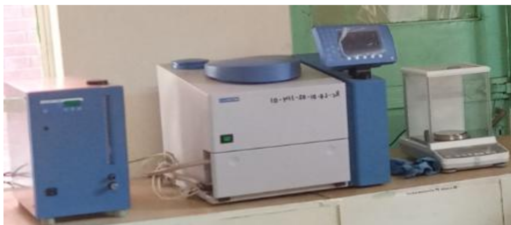
Figure 11: Bomb calorimeter used for raw and torrefied sample analysis
