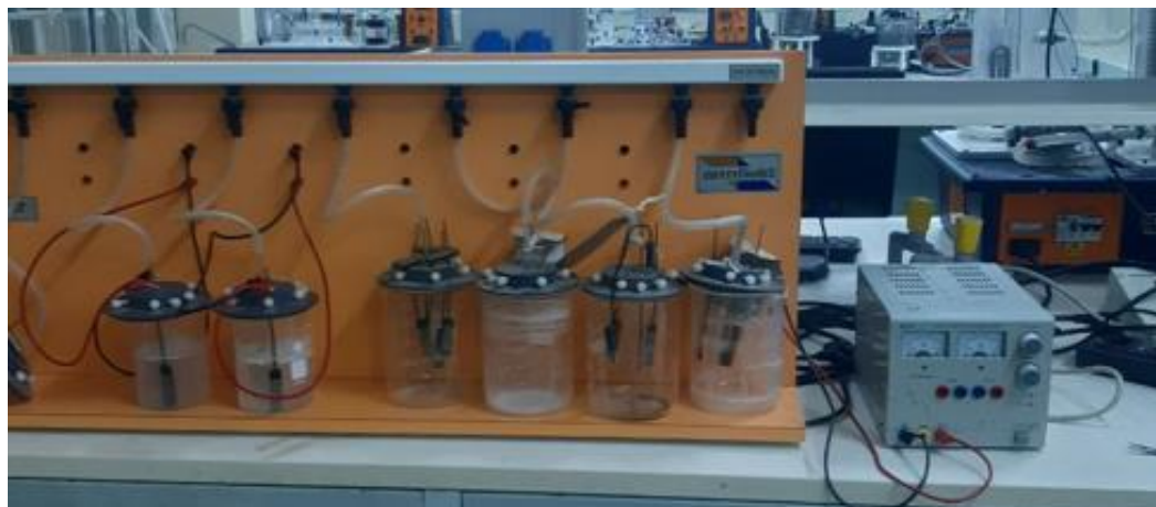
Figure 3. 7. Experimental setups of electrocoagulation
