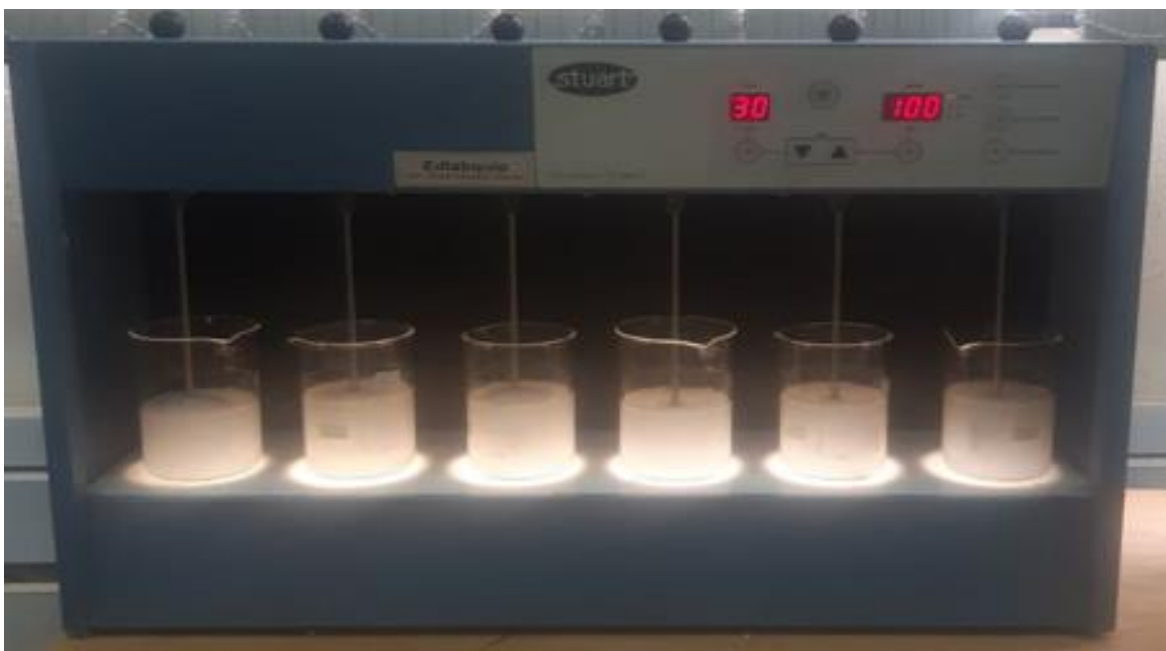
Figure 3. 5. Experimental setups of Jar test apparatus
