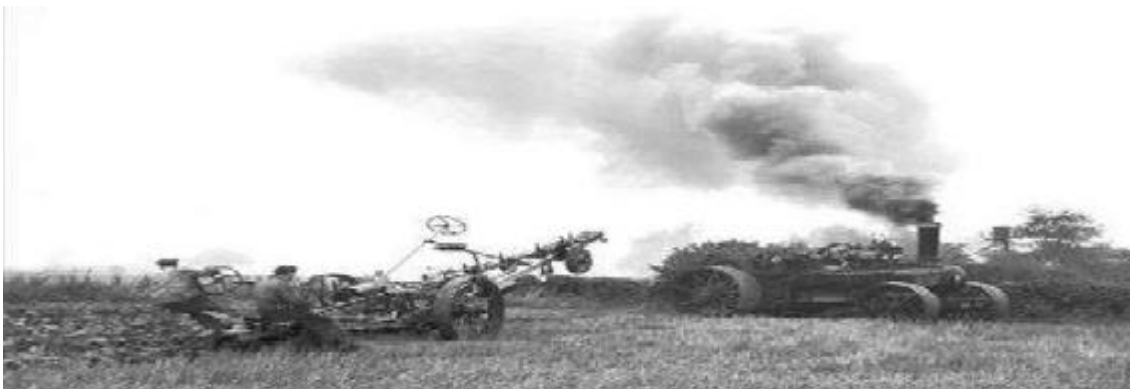
Figure 1. 1. Fowler’s traction engine pulling a plough (Source: Steam Plough Club, www.steamploughclub.org.uk/pictures.htm )
