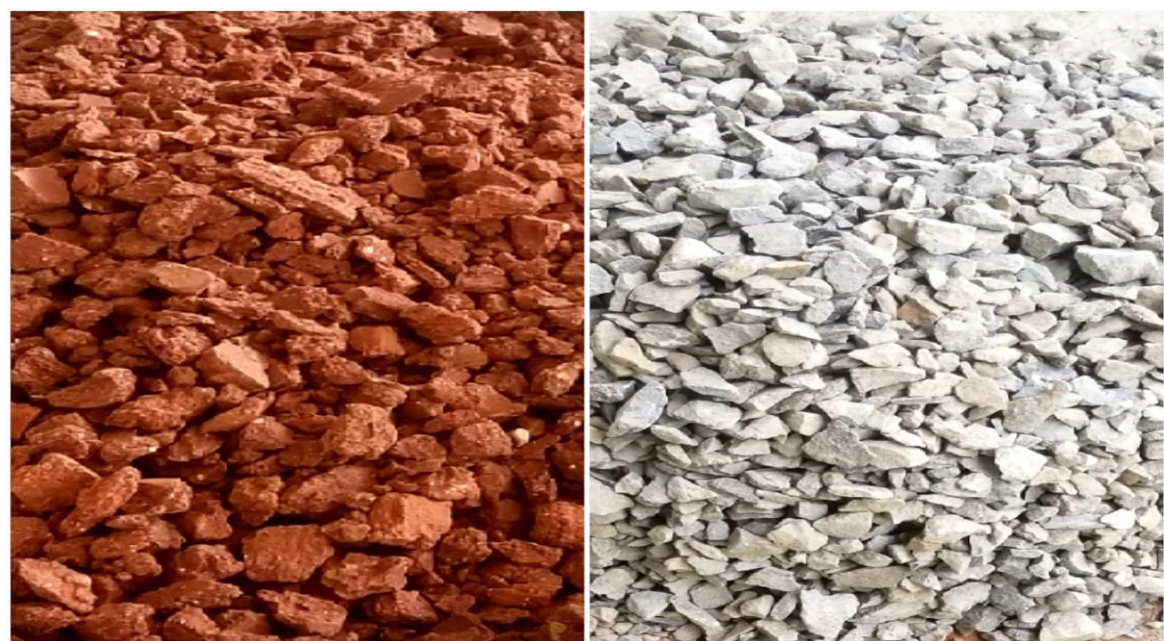
Figure 3.1 Waste clay bricks and natural coarse aggregates.
