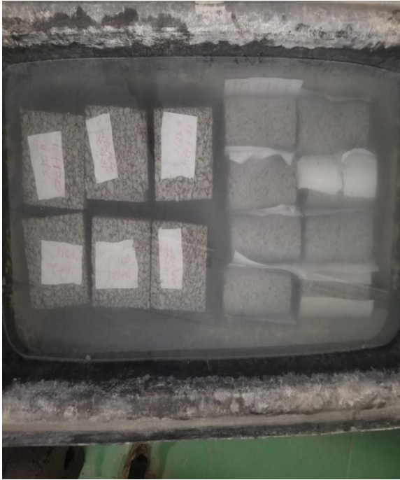
m) PC specimens in curing tank
