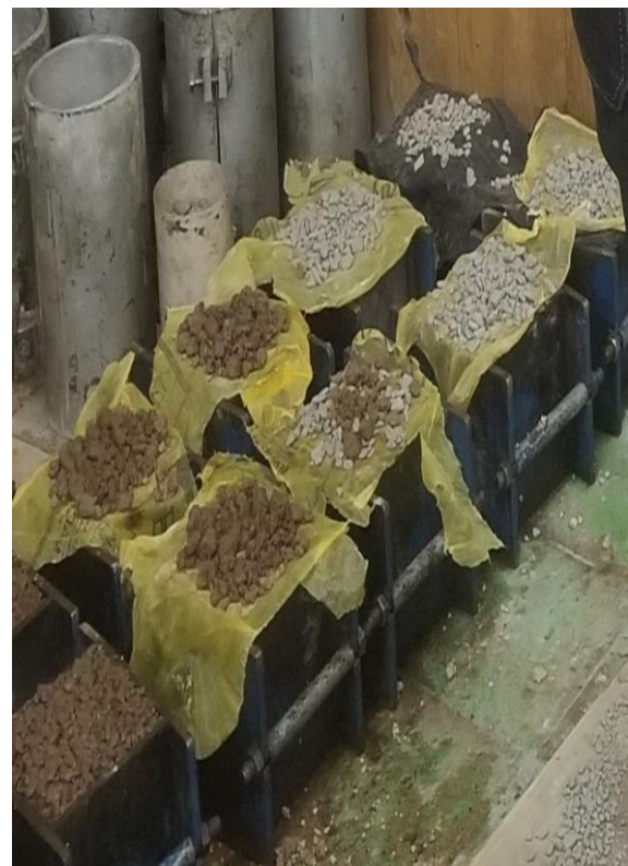
l) PC specimens covered with plastic sheet
