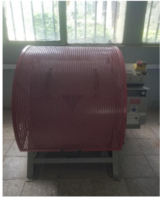
f) Set up of ALAV testing apparatus
