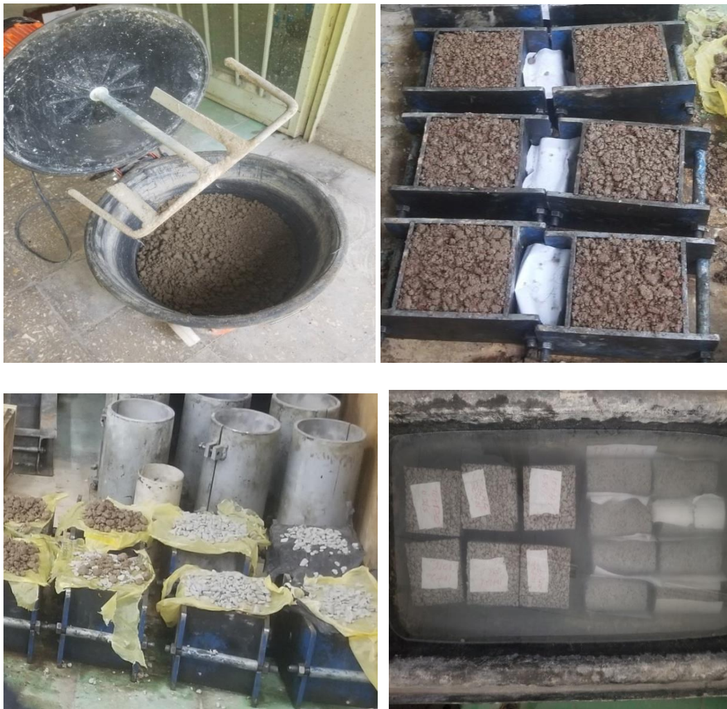
Figure 3.8 Casted pervious concrete molds.
