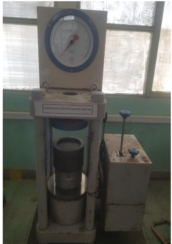
h) Set up of ACV testing apparatus
