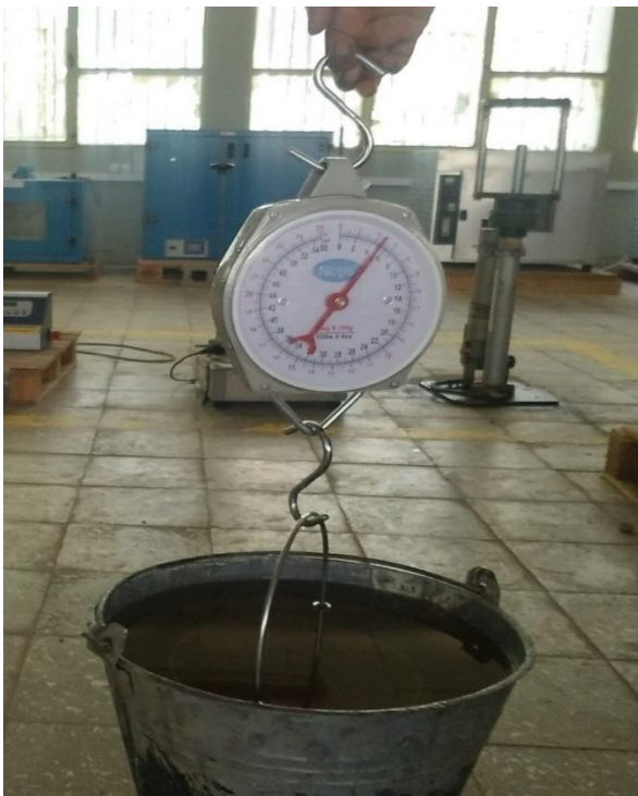
c) Specific gravity determination of WCBA
