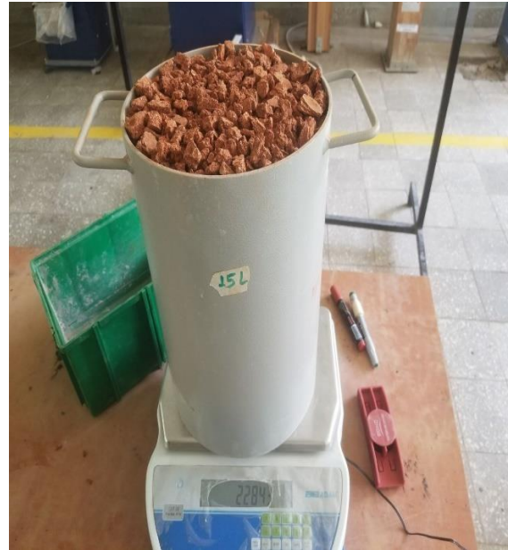
b) Unit weight determination of WCBA
