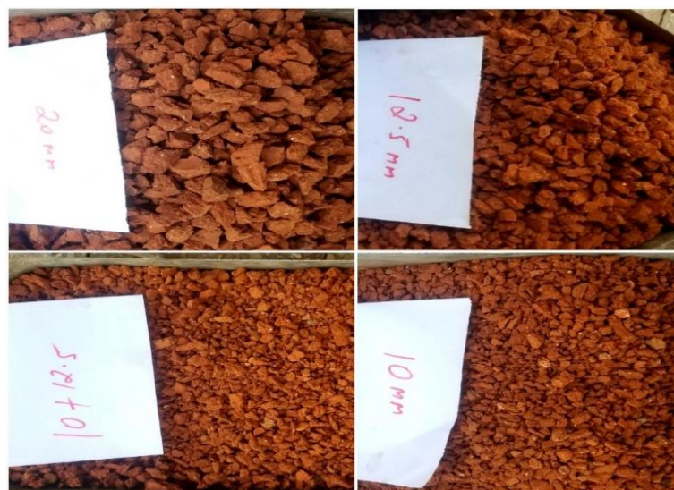
Figure 3.5 Crushed waste clay bricks aggregates of different sieve sizes.
