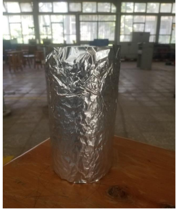
n) cylinder specimens ready for permeability test
