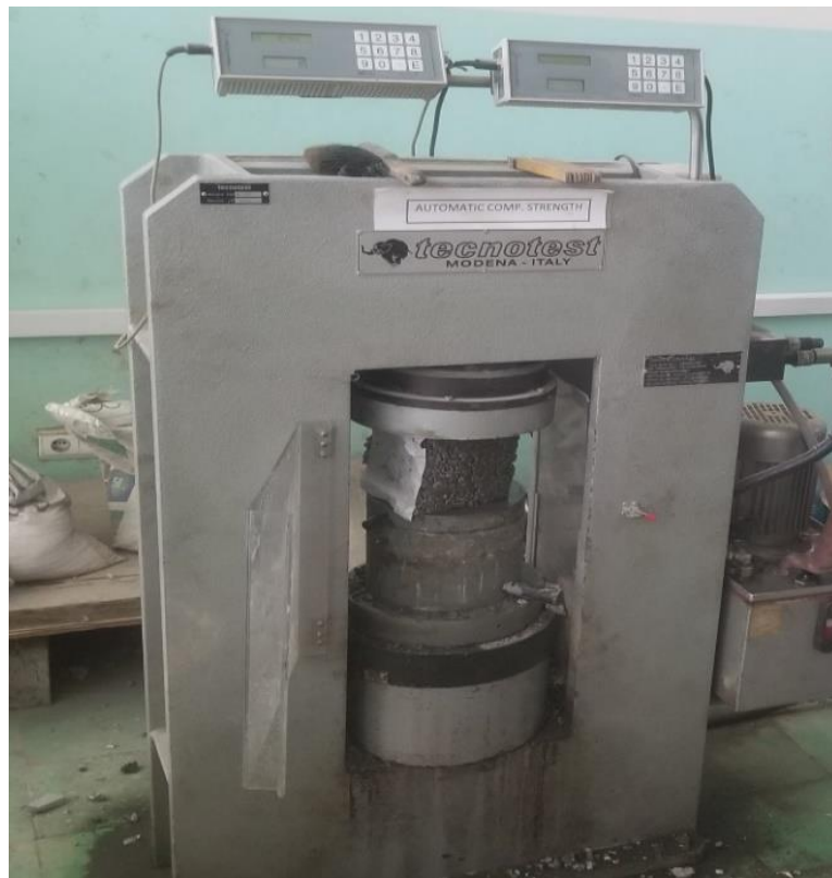
Figure 3.9 PC specimen in compression test machine
