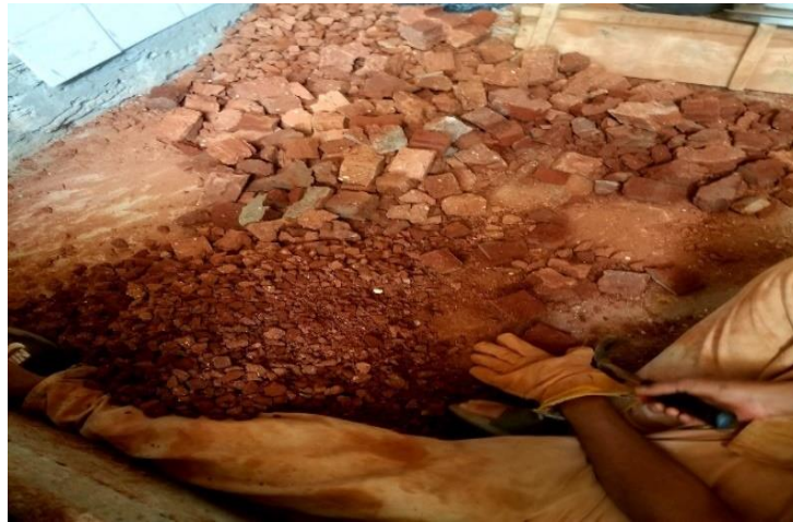
Figure 3.4 Size of manually crushed waste clay brick.
