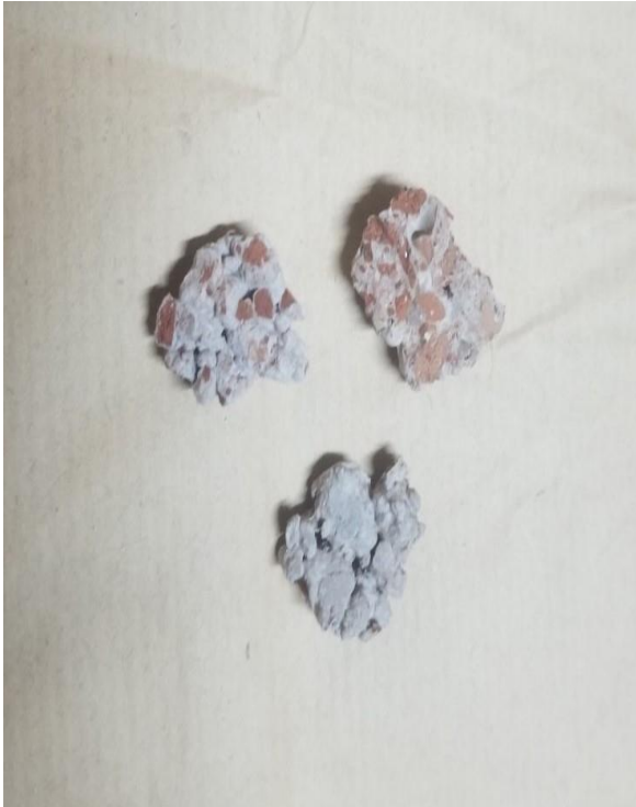
p) specimens ready for SEM test
