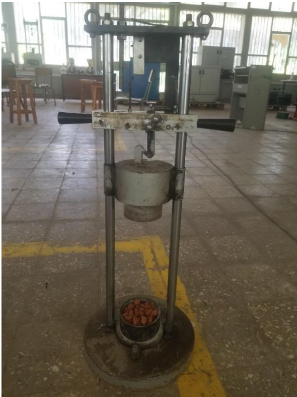
g) Set up of AIV testing apparatus
