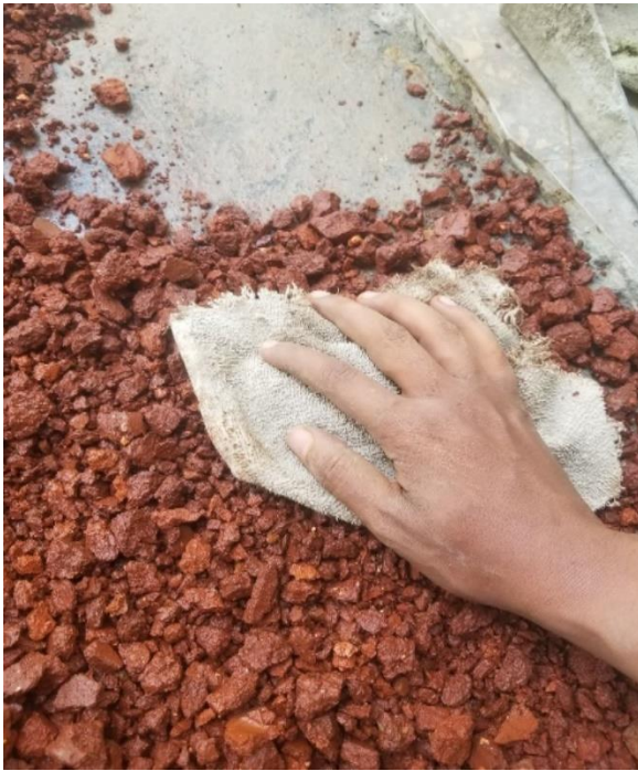
i) WCBA at SSD ready for mix
