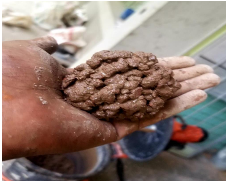
Figure 3.6 The consistency of the PC mixture.
