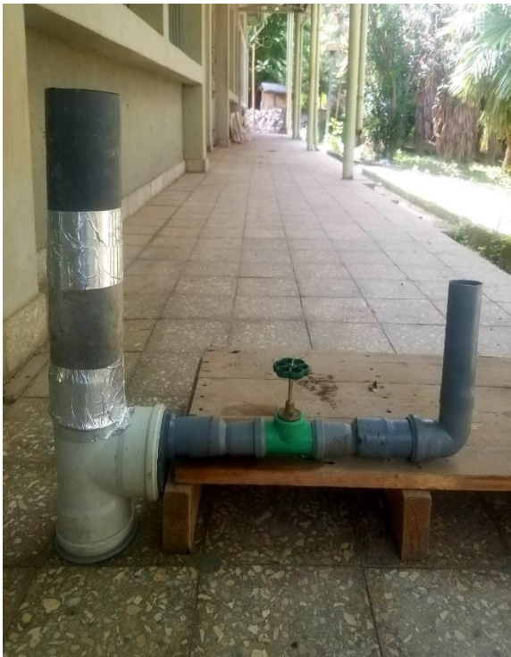
o) Set up of permeability testing apparatus
