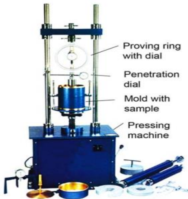
Figure 3.16 CBR testing equipment
