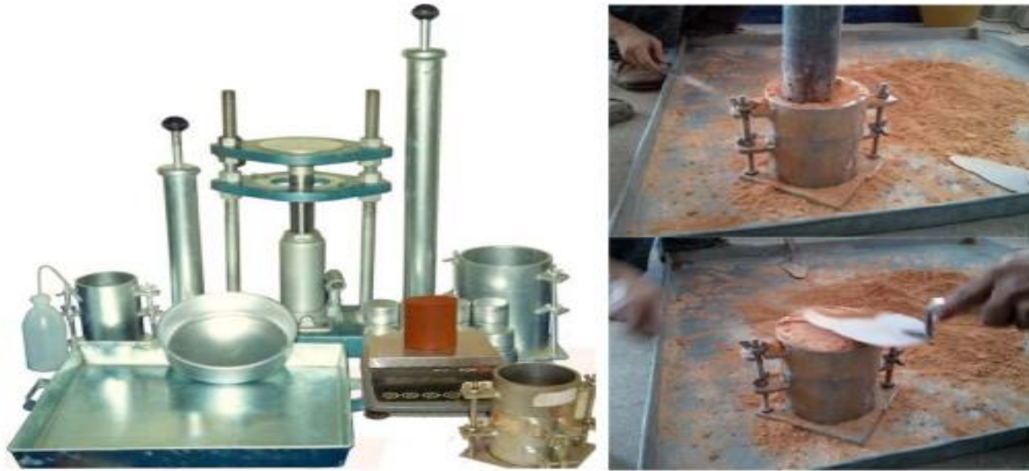
Figure 3.14 compaction testing materials
