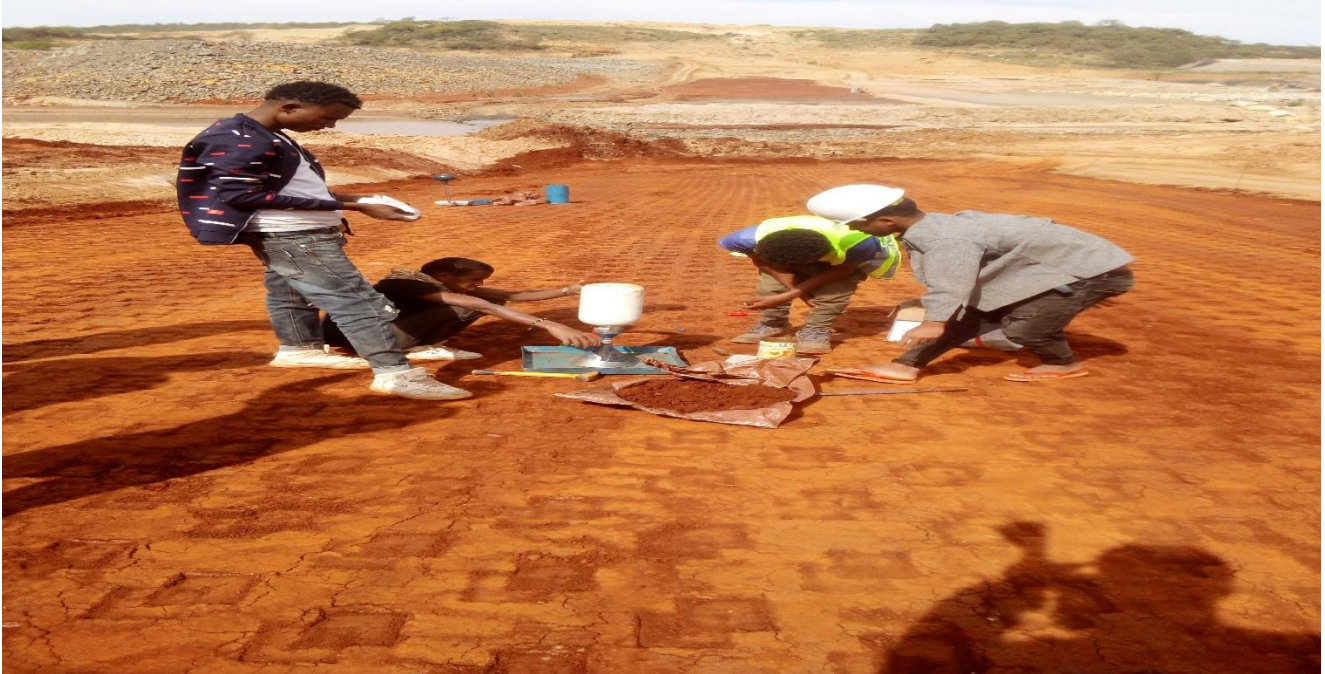
Figure 3.8: Clay core material compaction test conducted
