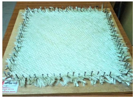
Figure 3.11: \pm 45^{\circ} of woven sisal fiber.
