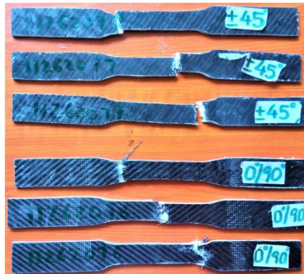
Figure 4.1: Fractured specimens after tensile test.
