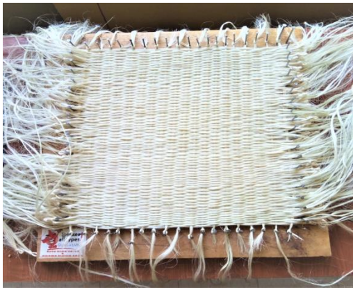
Figure 3.10: 0^{\circ}/90^{\circ} of woven sisal fiber.
