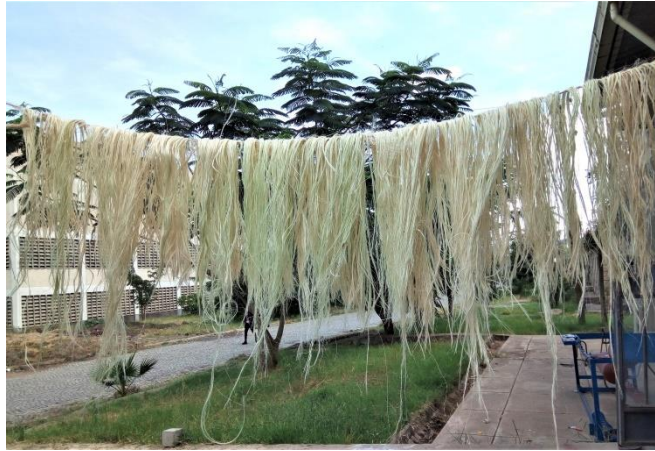
Figure 3.9: Drying sisal fiber in sun light.
