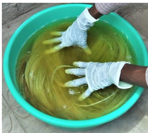
Figure 3.8: Soaking the sisal fiber in base solution.
