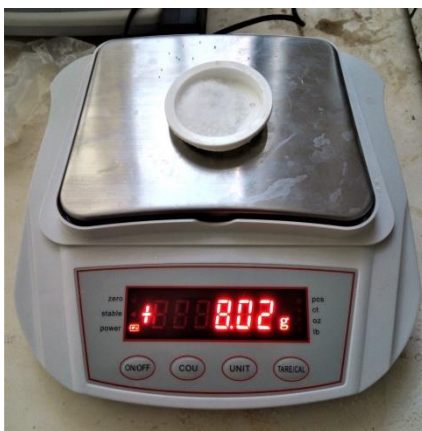
Figure 3.7: Measurement of NaOH using digital balance.
