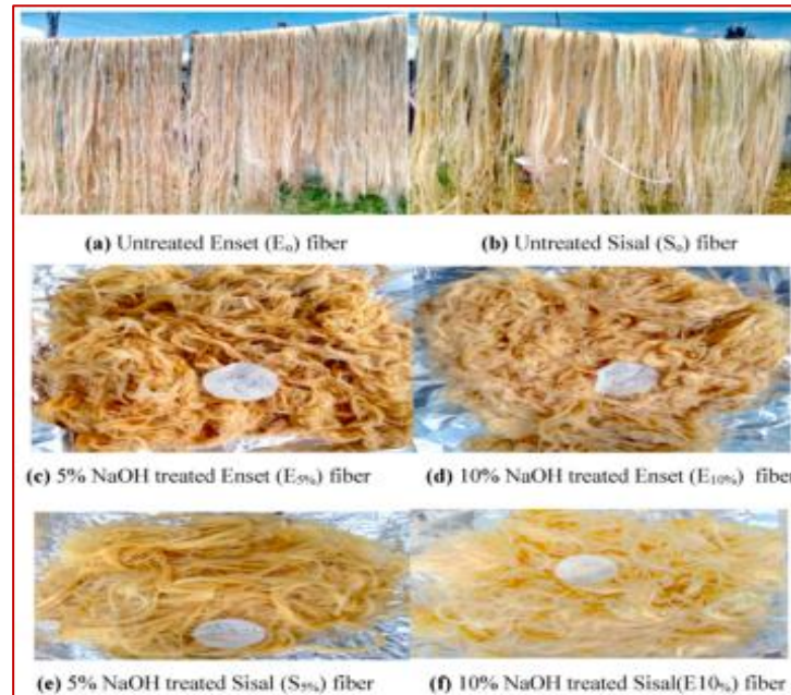
Figure 3. 2 Untreated and treated with 5% and 10% NaOH of enset and sisal fibers
