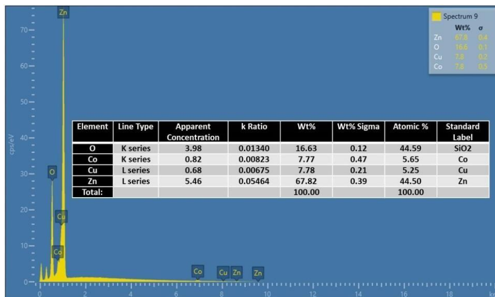
Figure 12. Image analysis using scanning electron microscopy (SEM): (a) the SEM image of ZnO NPs and 1% and 20% BNCs and TNCs. The nanocomposites showed greater porosity compared to the ZnO NPs. (b) The EDX analysis for the 20% TNCs; the inset table in the EDX image is the detailed compositional analysis.
