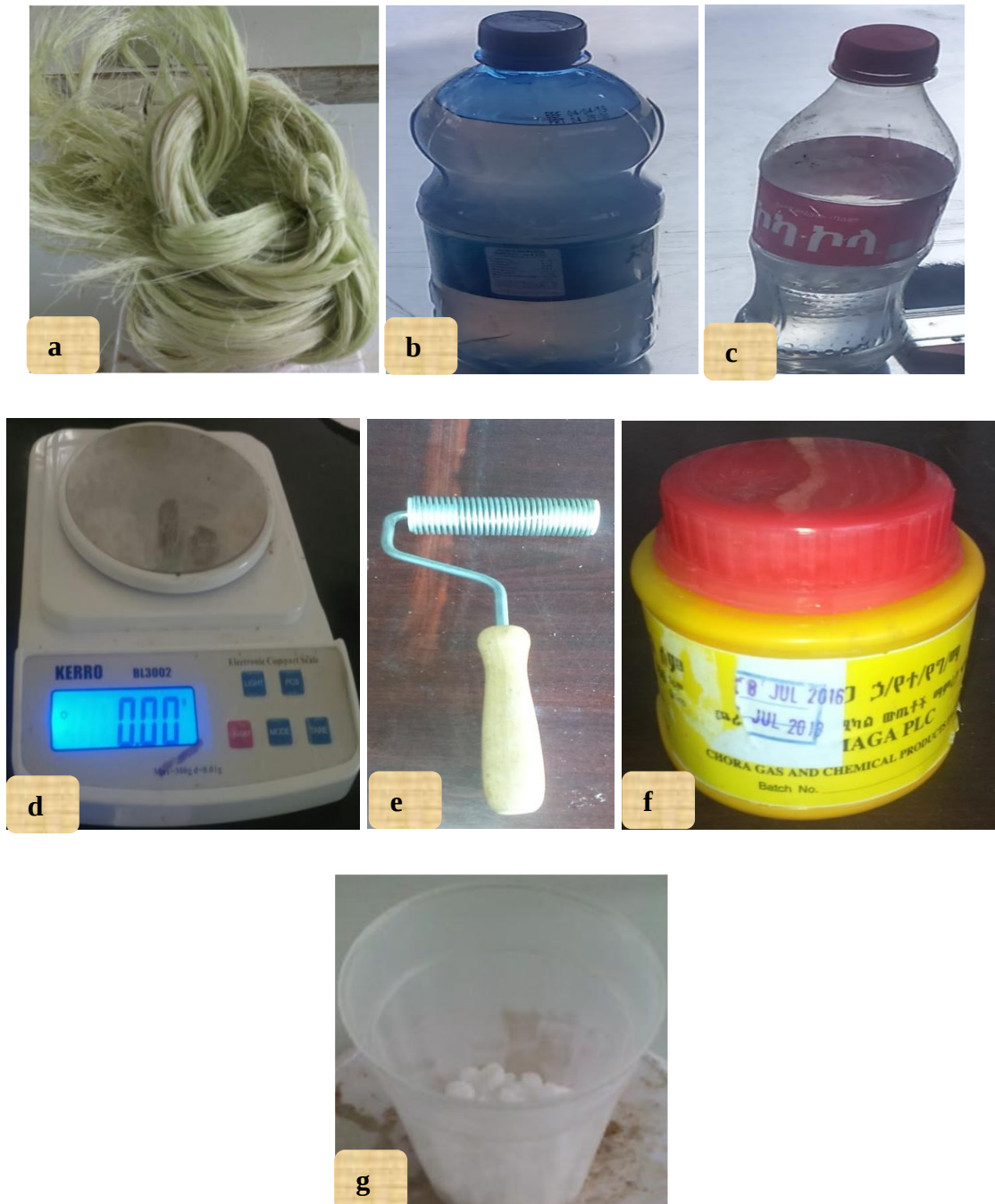
Figure 3. 1 Materials used: (a) extracted sisal fiber (c) polyester resin (c) hardener (d) electronic balance (e) roller (f) release wax (g) Sodium Hydro Oxide
