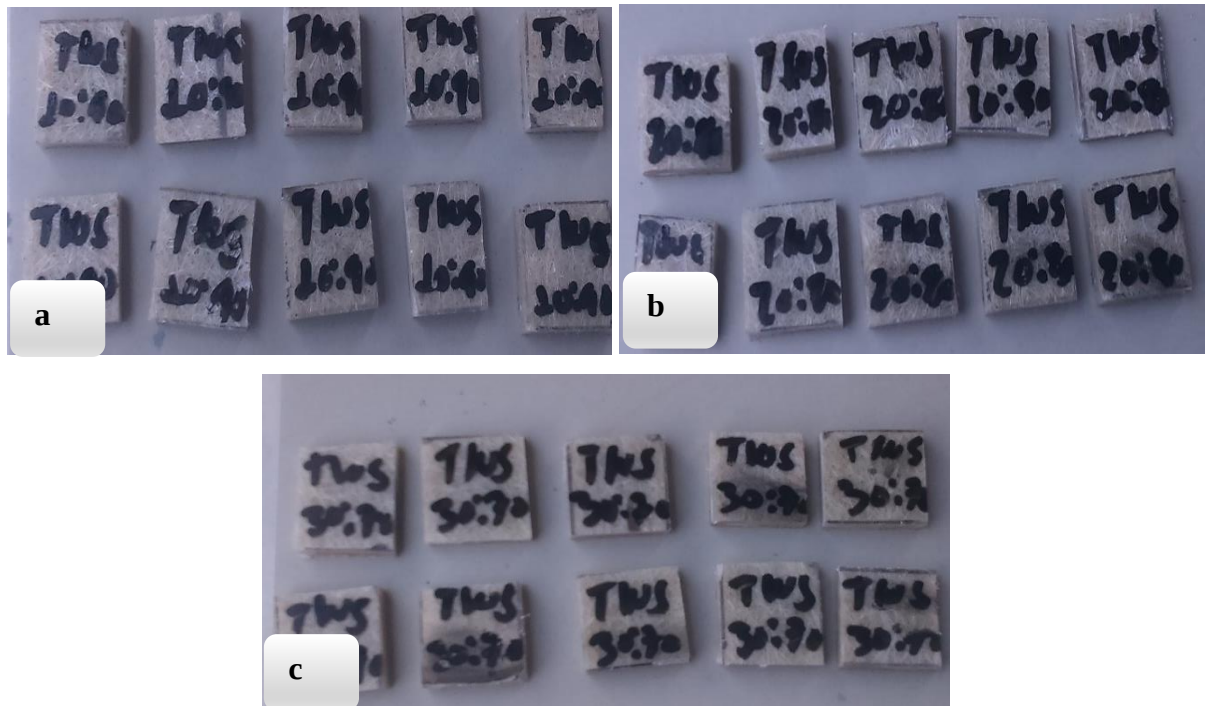
Figure 3. 30 Treated fiber water absorption test specimen: (a) 10% fiber and 90% matrix, (b) 20% fiber and 80% matrix, and (c) 30% fiber and 70% matrix
