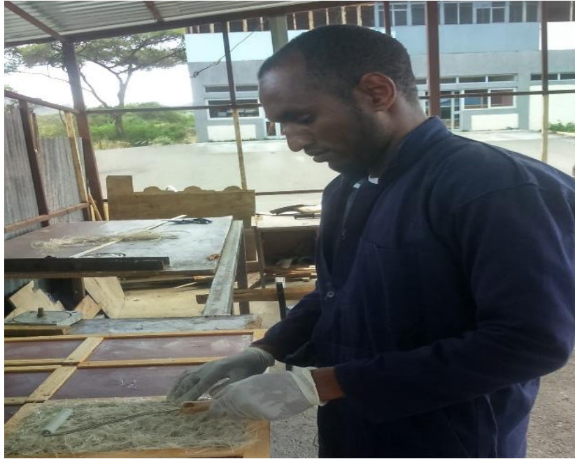
Figure 3. 11 Preparation of SFPCM by Hand Layup Method
