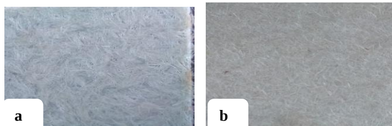
Figure 3. 14: (a) Untreated sisal fiber composite samples (b) Treated sisal fiber composite sample
