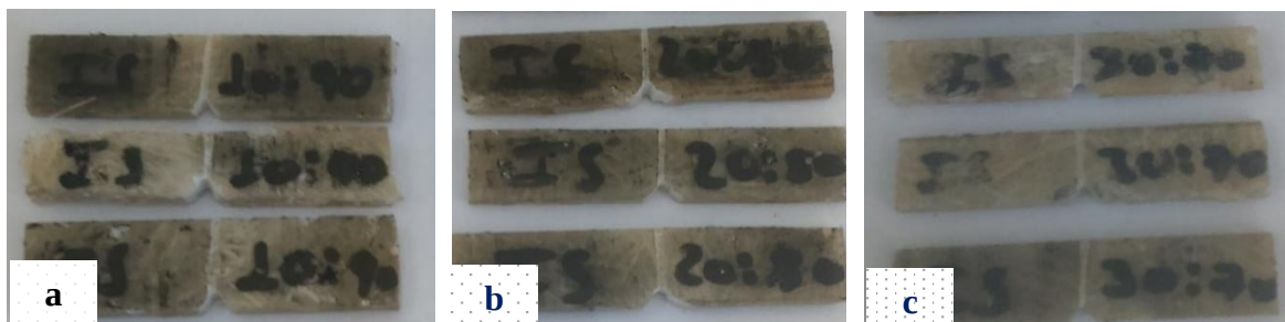
Figure 3. 25 Untreated fiber impact test specimen: (a) 10% fiber and 90% matrix (b) 20% fiber and 80% matrix (c) 30% fiber and 70% matrix
