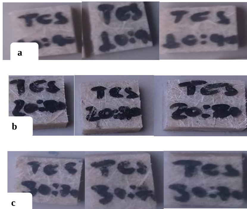
Figure 3. 22 Treated sisal fiber compressive test specimens: (a) 10% fiber and 90% matrix, (b) 20% fiber and 80% matrix, and (c) 30% fiber and 70% matrix
