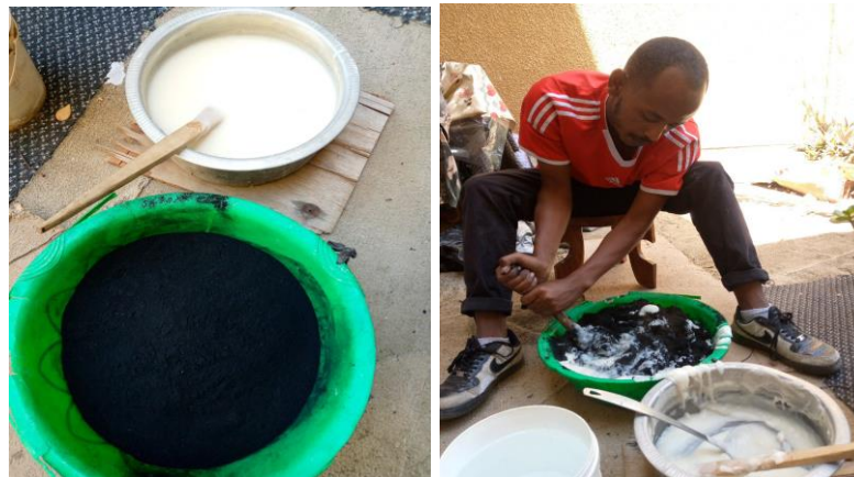
Figure 5:6 Mixing powder carbonized coffee husk with binder
