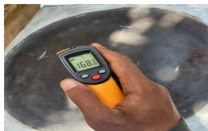
Figure 6:9 Measuring surface temperature of mitad using infrared thermometer
