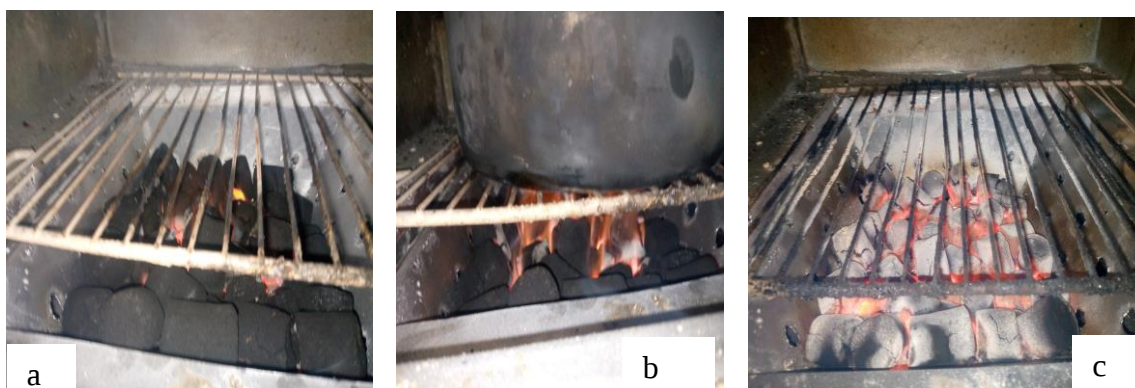
Figure 6:4 Combustion of briquette a) ignition stage b) flaming combustion c) smoldering combustion
