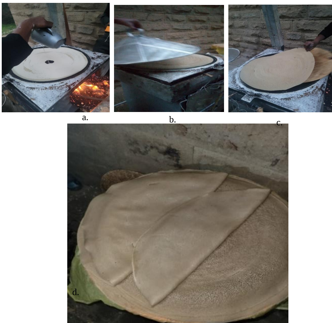
Figure 6:12 Injera baking test a) pouring of batter b) closing the lid cover c) after the batter baked (took out) d) quality injera baked
