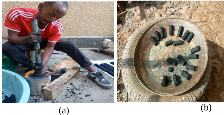
Figure 5:7 Molding and Drying a) molding coffee husk bio-briquette b) briquette drying under sun
