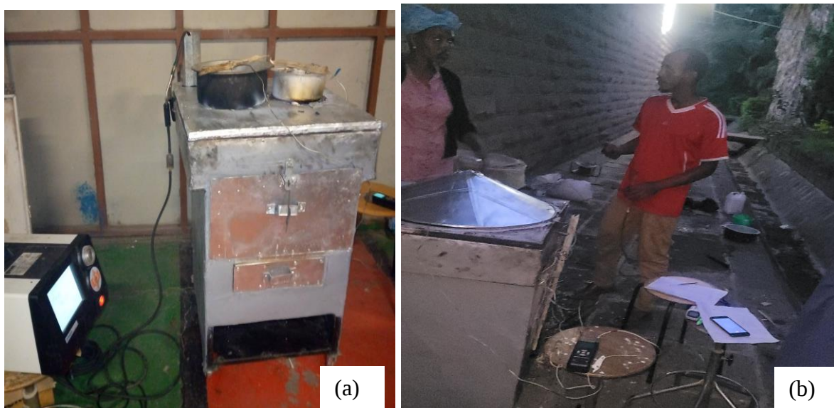
Figure 5:8 Experimental setup during a)water boiling test b) injera baking
