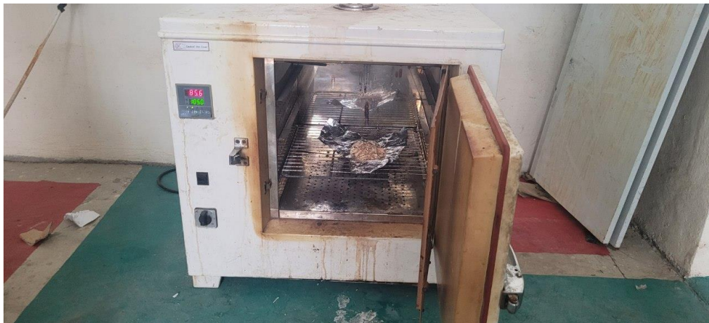
Figure A5: 2 Sawdust sample in oven for moisture content test
