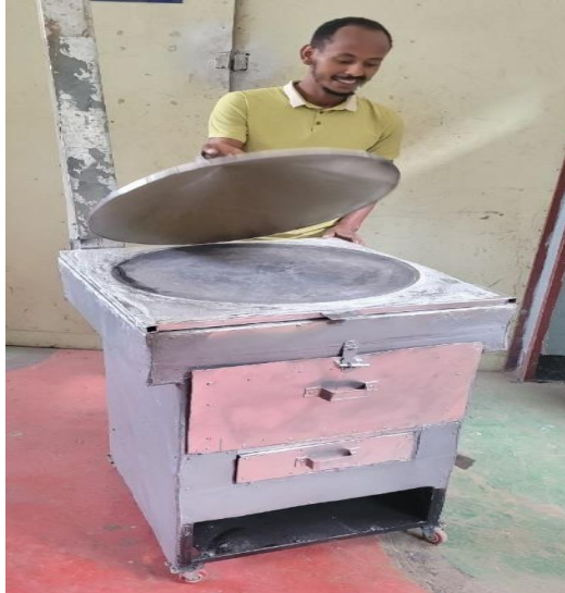
Figure 5:2 Multipurpose stove when baking pan is assembled
