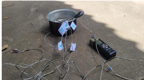
Figure A3: 1 Thermocouple calibration using boiled water
