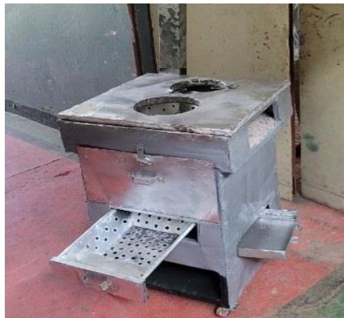
Figure 5:3 Multipurpose stove when cooking part is assembled
