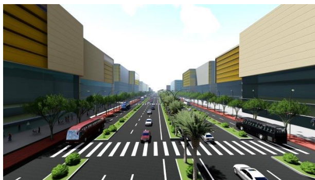
Figure 4.4.15: Separated transportation lane (PAS)
