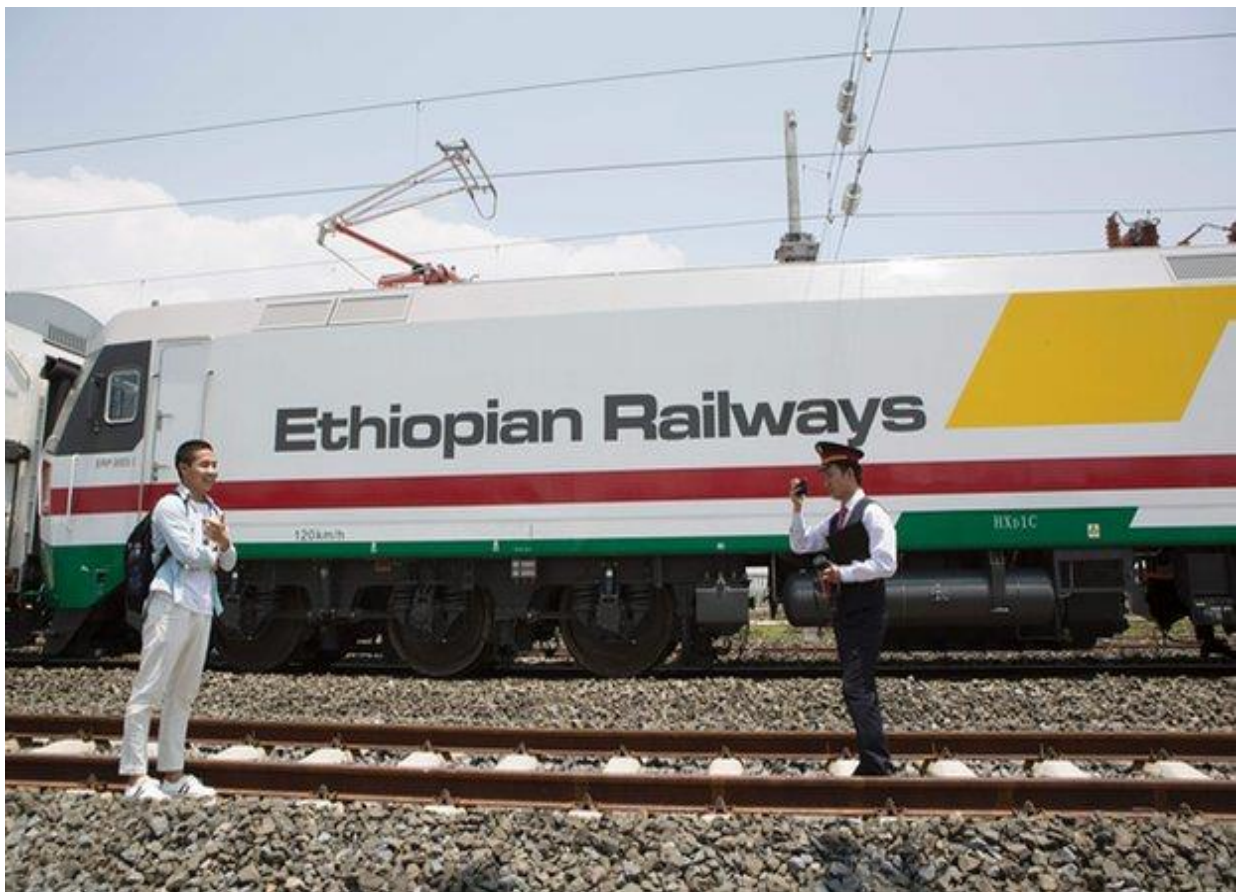
Figure 10: This Ethiopian train using overhead or catenary wire suspended from poles along the track.
