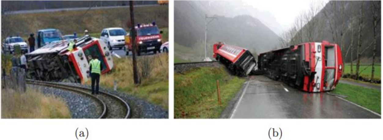
Figure 13: Rollover accidents of rail vehicles, (a) on curved track at Uttendorf (Austria) in 2002, (b) on tangent track at Wasserauen (Switzerland) in 2007 [18].
