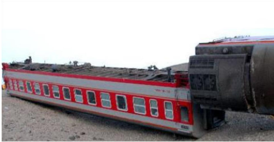
Figure 1: Driving train overturned by crosswinds.
