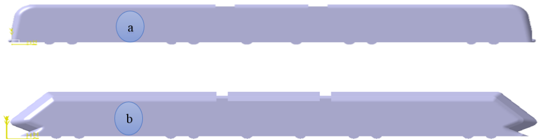
Figure 28: Ethiopian Light Railway Transit Aerodynamic shape of nose Figure a is Existing and b is Optimized Models.
