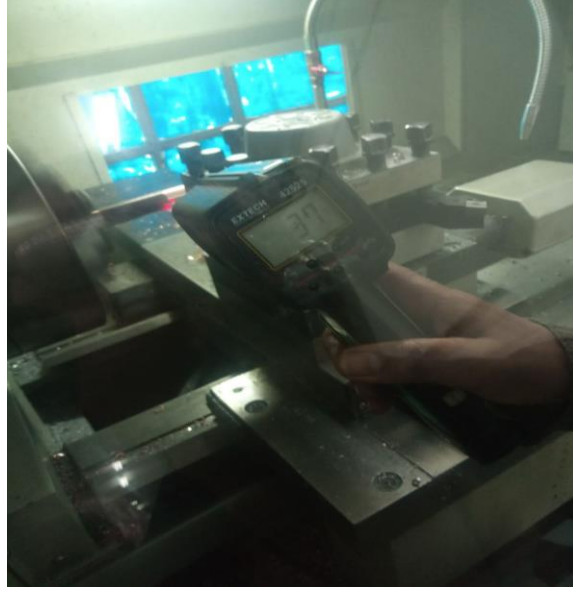
Figure 3.9: Measurement of Tool-work piece interface Temperature
