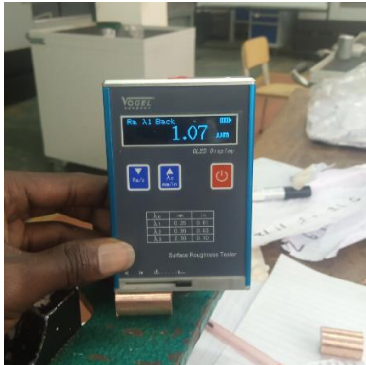
Figure 3.8: Measurement of surface roughness
