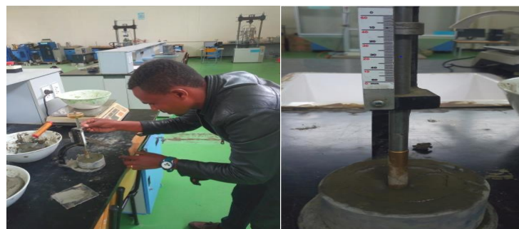
Figure 3-1 Normal consistency of cement (Appendices H2)
