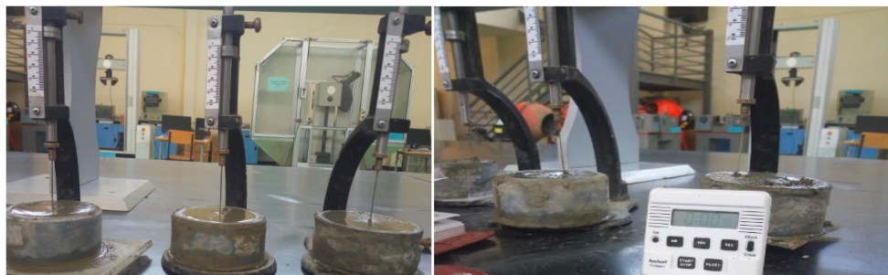
Figure 3-2 Setting time of hydraulic cement (Appendices H3)
