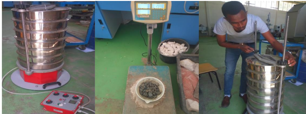
Figure 3-5 Coarse aggregate gradation (Appendices N)
