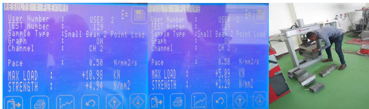
Figure 4-6 Results of flexural Strength of concrete results (Appendices J)
