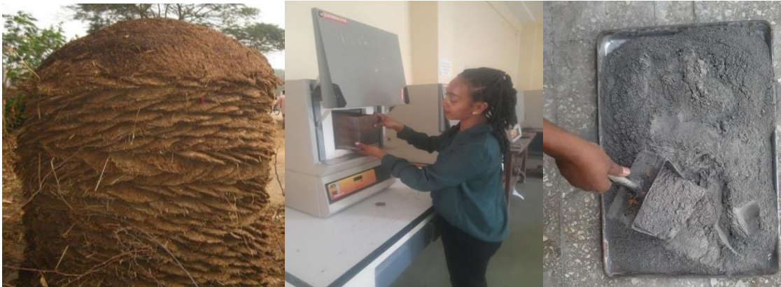
Figure H-1 sun dried cowdung, furnace and cow dung ash
