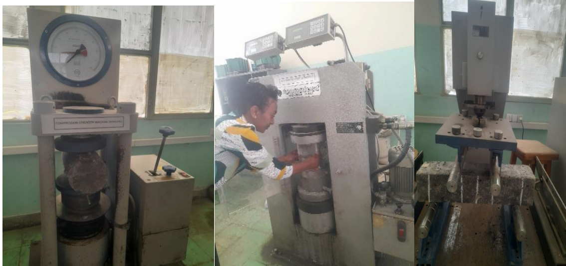
Figure H 7 : tensile ,compressive and flexural strength test conducting
