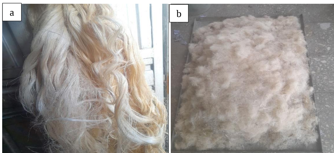
Figure 3. 6 : (a) Enset ventricosum fiber and (b) copped enset fiber
