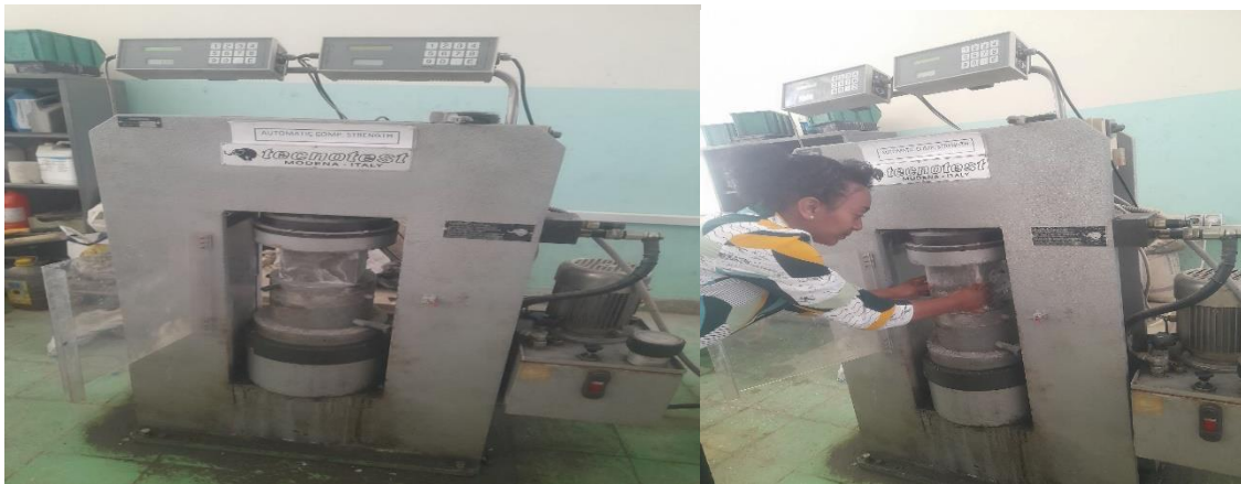
Figure 3. 11: Compressive strength test
