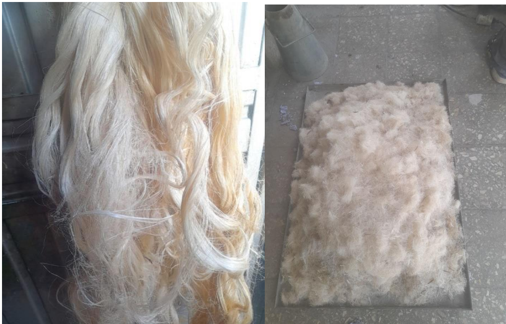
Figure H 8 Enset fiber and chopped enset fiber
