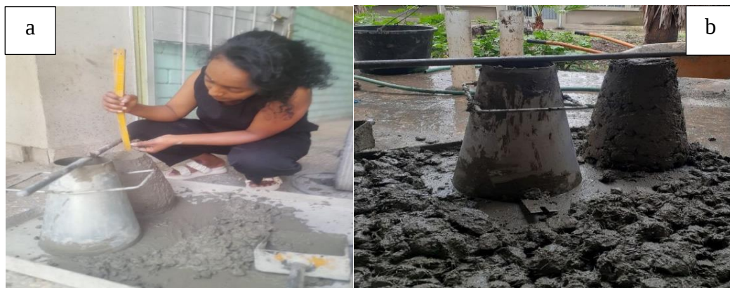
Figure 3. 8: Workability test a) conventional concrete b) Modified concrete
