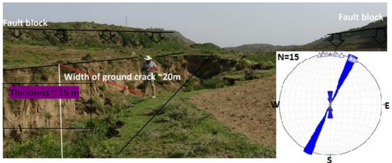
Figure 15: Showing ground crack orientation relationship with faults attitude.
