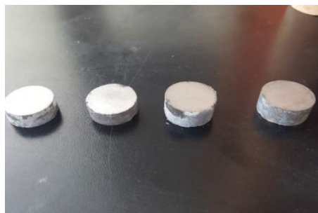
Figure 3.1 Sintered pure Mg and Mg-Ta-HA composites fabricated through powder metallurgy process.
