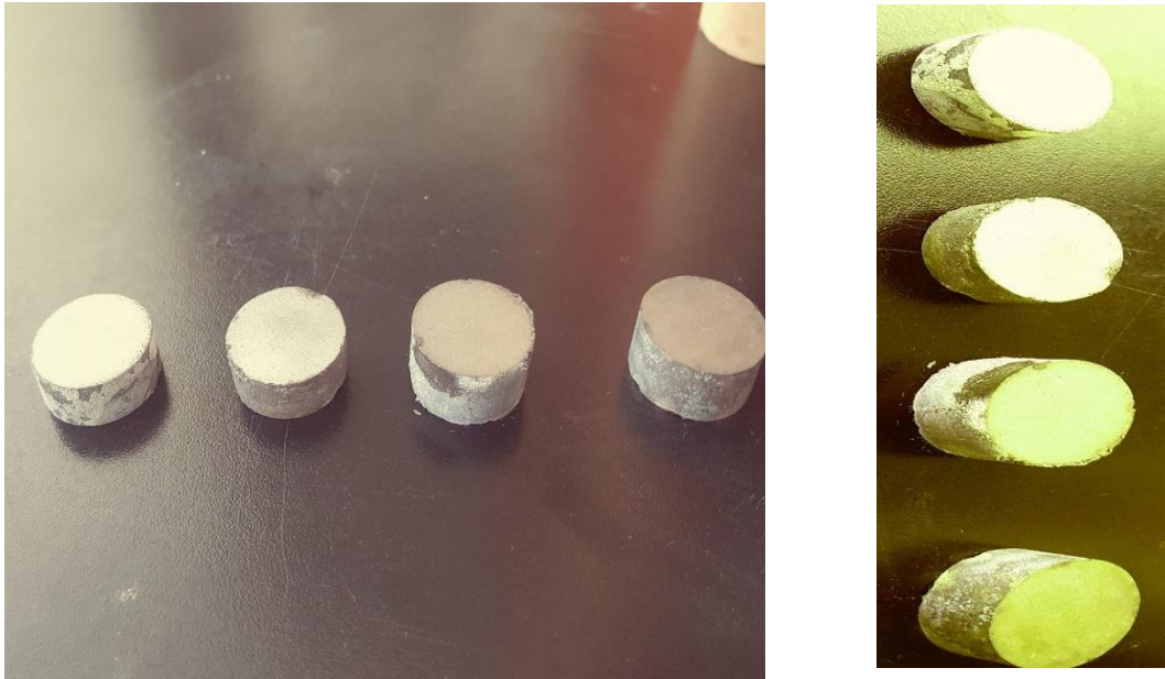
Figure 2.4 Sintered samples at different wt% reinforcement
