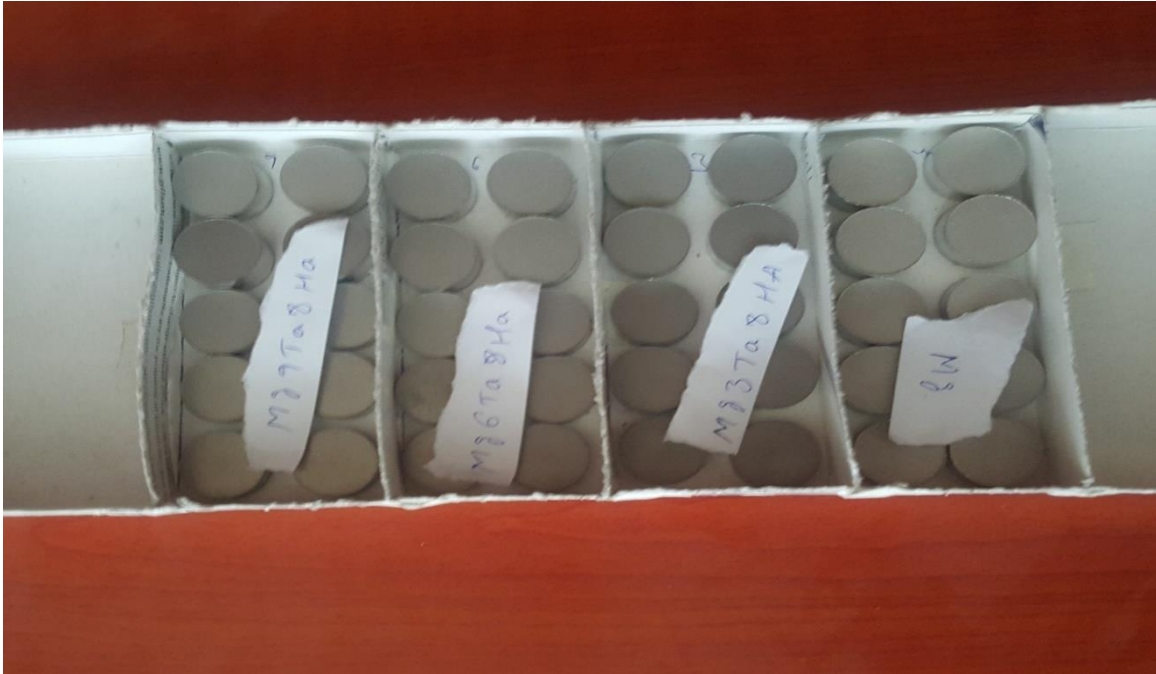
Figure 2.2 Compacted green body at different composition
