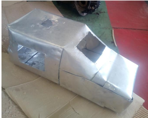
Figure 4.9: Model of the car cabin fabricated from aluminum sheet metals
