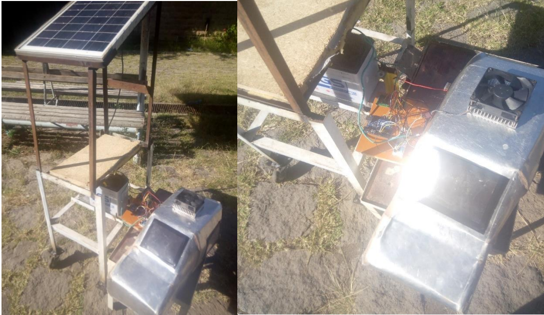
Figure 4.12: Demonstration test for the thermoelectric cooling system
