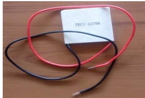
Figure 4.2: Peltier's TEC module
