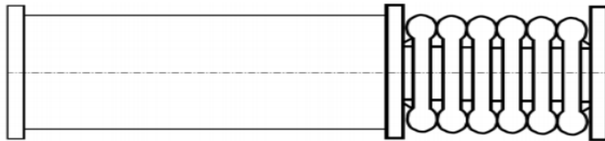
Figure 2.1: Axial collapse mode
