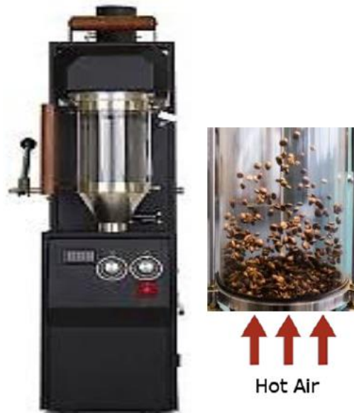
Figure 2.4: Fluidized Bed Roasting of Coffee (Kelly, 2018)
