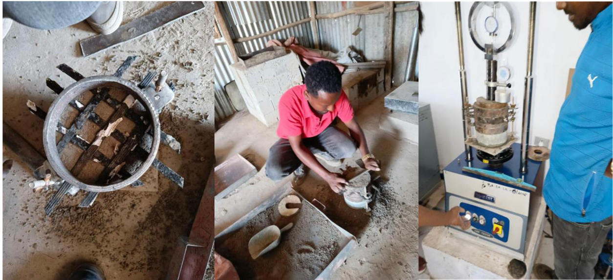
Figure 3.3: Reinforcement and anchoring of the first layer geogrid inclusion on CBR Mould
