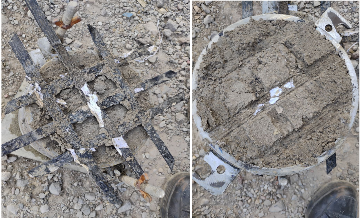
Figure 5.13: Deformation reduction potential of geogrid material while reinforced on CBR Mould
