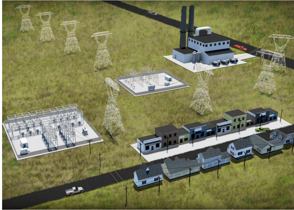
Figure 2.1: Transmission and distribution grid structure within the power industry [33]
