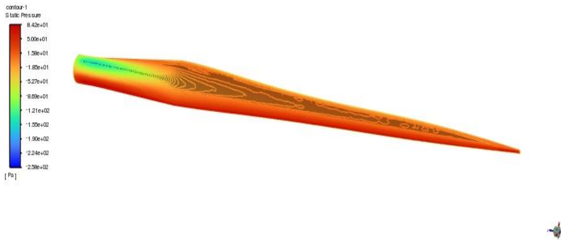
Figure 4-48 Pressure contour at \alpha = 15^\circ
