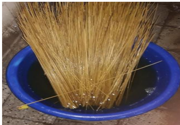
b) Bamboo fiber soaked in sodium hydroxide
