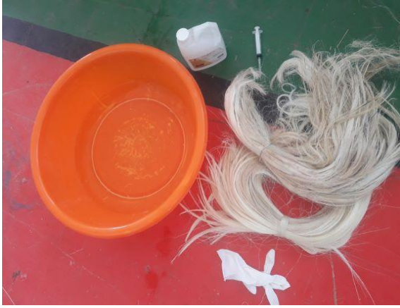
(a) Preparation of alkaline solution
