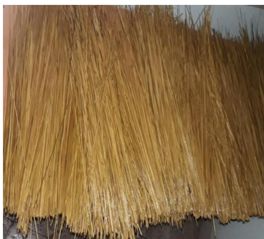
c) Alkaline treated bamboo fiber
