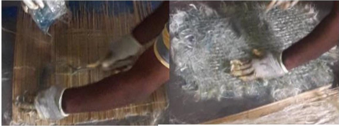
(f) Moving roller brush in fiber resin layer
