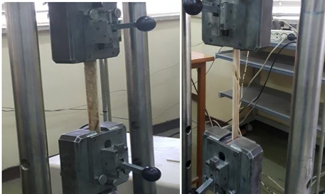
Figure 3.28: UTM machine Sample loaded condition for tensile testing
