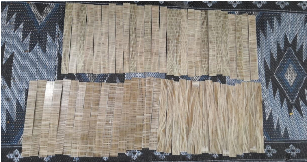
Figure 3.18: Cutting of sample specimen using splitter
