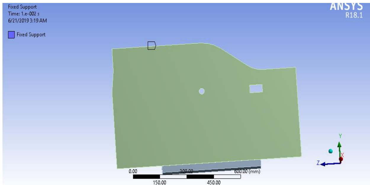
Figure 4.39: Applying boundary conditions on ANSYS Workbench
