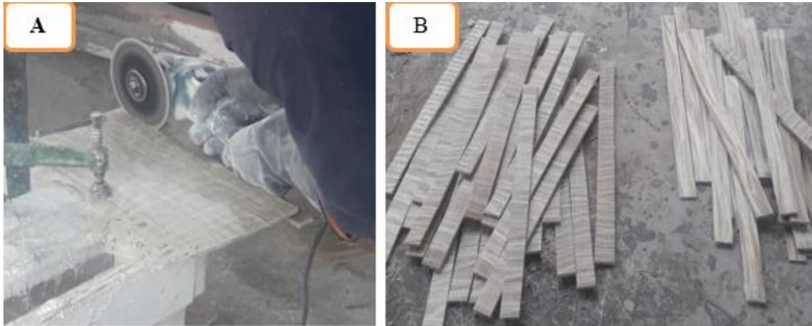
Figure 3.18: Cutting of sample specimen using splitter
