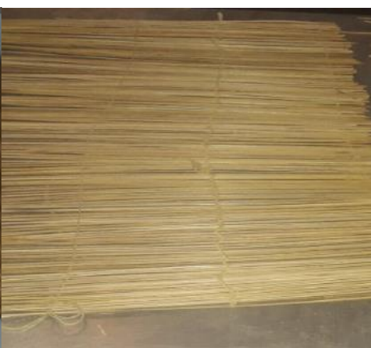
d) Unidirectional (UD) bamboo fiber with zero degree fiber orientation
