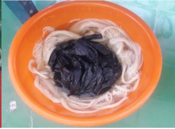
(b) Soaking sisal fiber in NaOH solution
