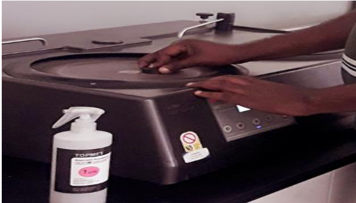
Figure 3.36: Polishing sample specimen
