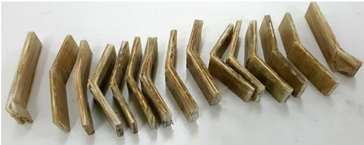
Figure 4.29: Fractured specimen after compression test
