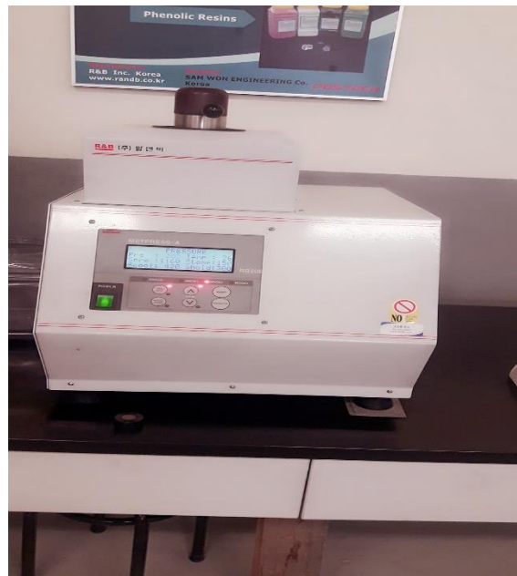
Figure 3.35: Mounting the sample in hot mounting press
