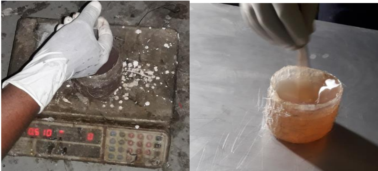
(a) Mixing of polyester resin and catalysts according to ratio
