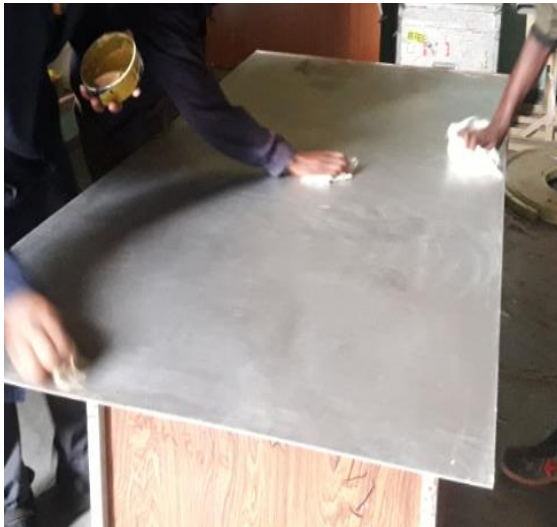
(c) Polishing of mold surface
