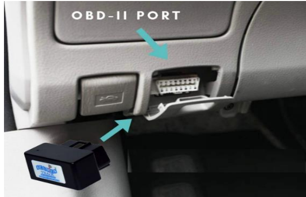
Figure 3.5: OBD II port for GPS installation
