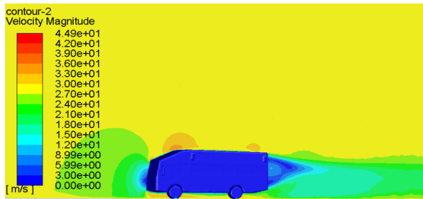
Figure 6.53: velocity contour of the modified bus at 100 km/hr
