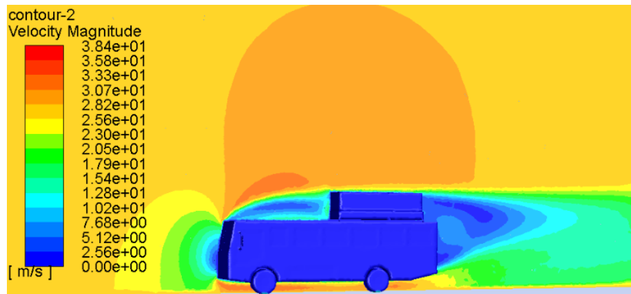
Figure 6.38: Velocity Contour of the baseline bus with luggage at 100 km/hr
