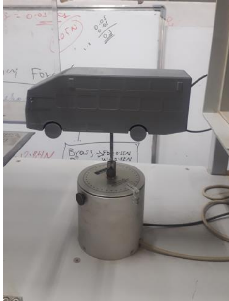
Figure 5.6: Securing the modified bus model in the wind tunnel
