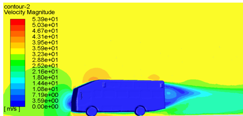
Figure 6.54: velocity contour of the modified bus at 120 km/hr
