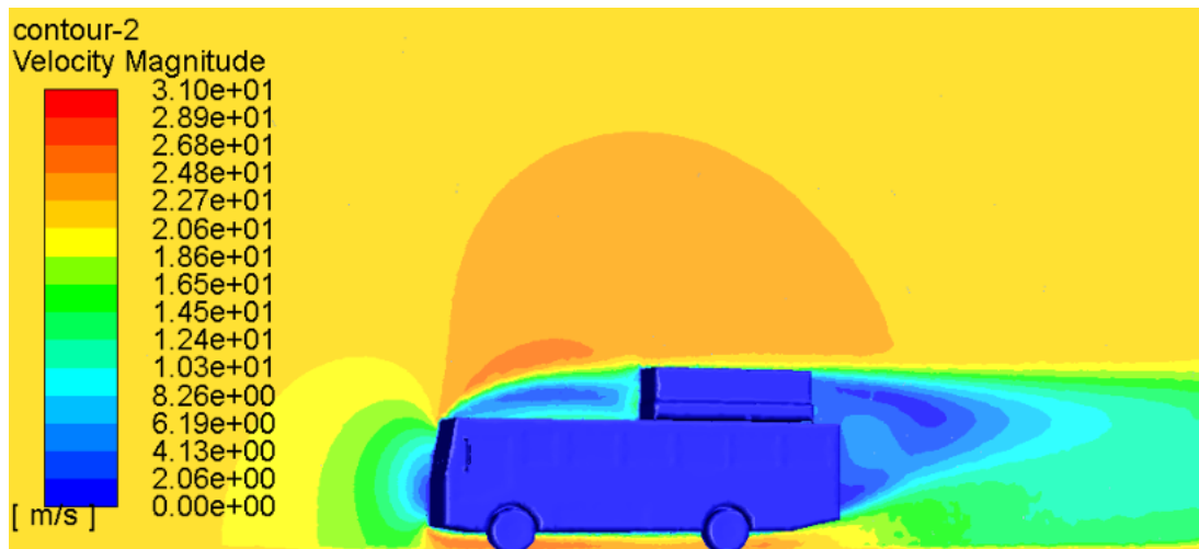
Figure 6.37: Velocity Contour of the baseline bus with luggage at 80 km/hr
