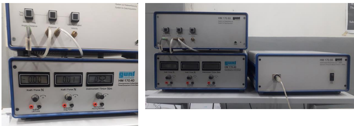
Figure 5.7: Zeroing the measuring equipment
