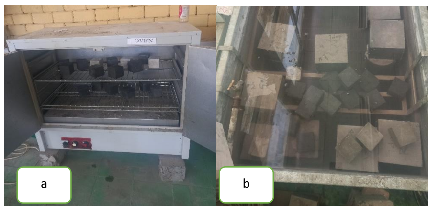
Figure 3. 14 Water Absorption test. Oven dry(a), submerged(b)
