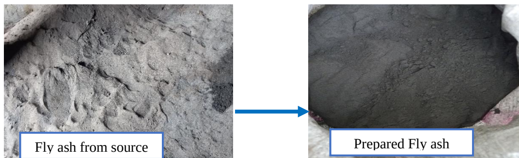
Figure 3. 2 Coal Fly Ash Preparation
