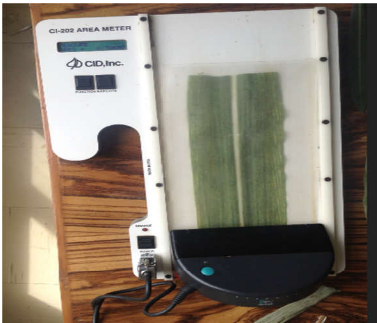
Figure 1: CI-202 area meter used in the leaf area measurement
