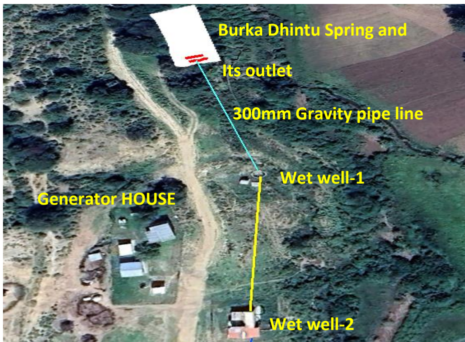
Fig 4: System components in source area
