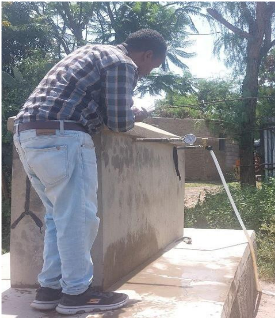
Annex-3: Photos taken while collecting Observed data of pressure at water points using pressure gauge
