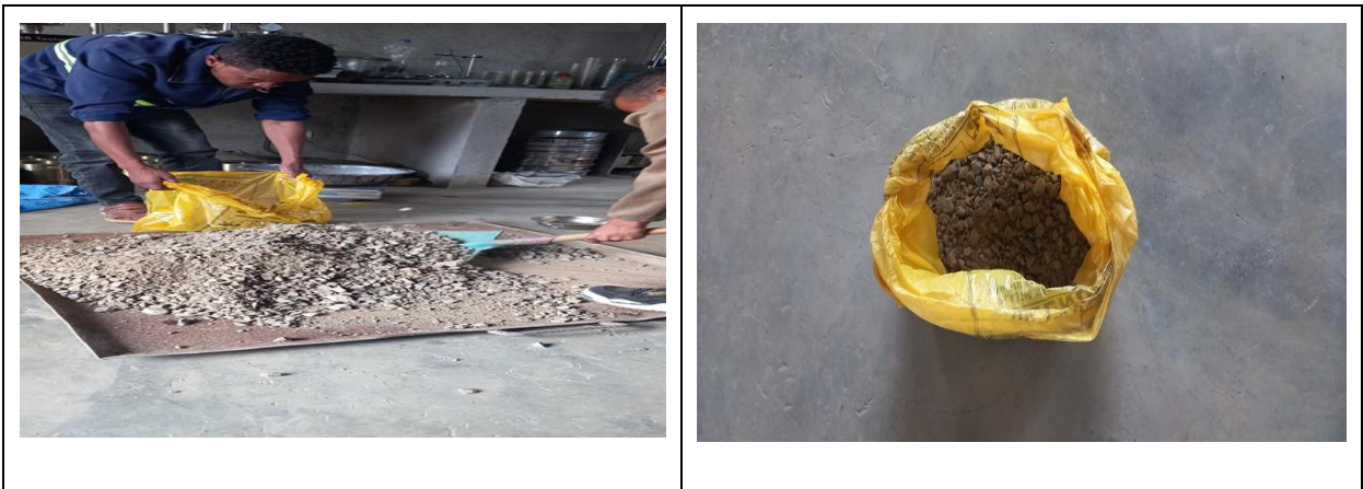
Figure 3.13 Sample Preparation for Crushed Aggregate Base Course
