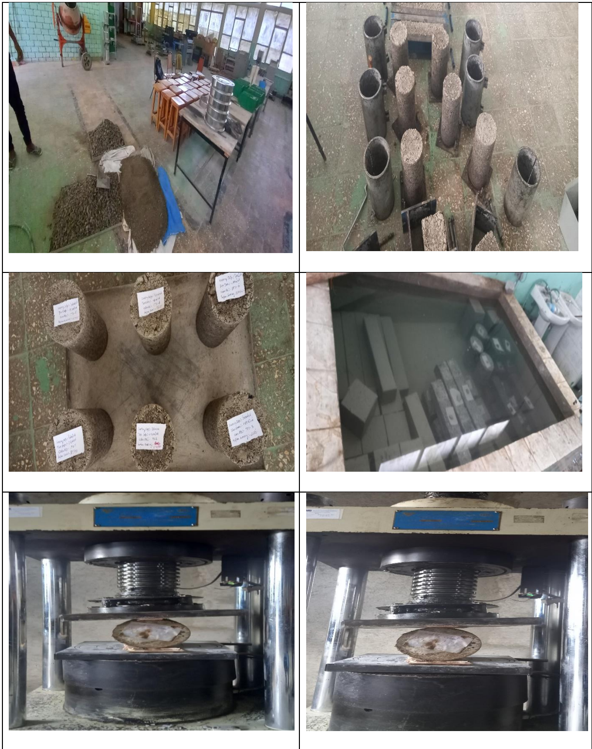
Figure 3.17 Indirect Tensile Strength test procedure for CTB
