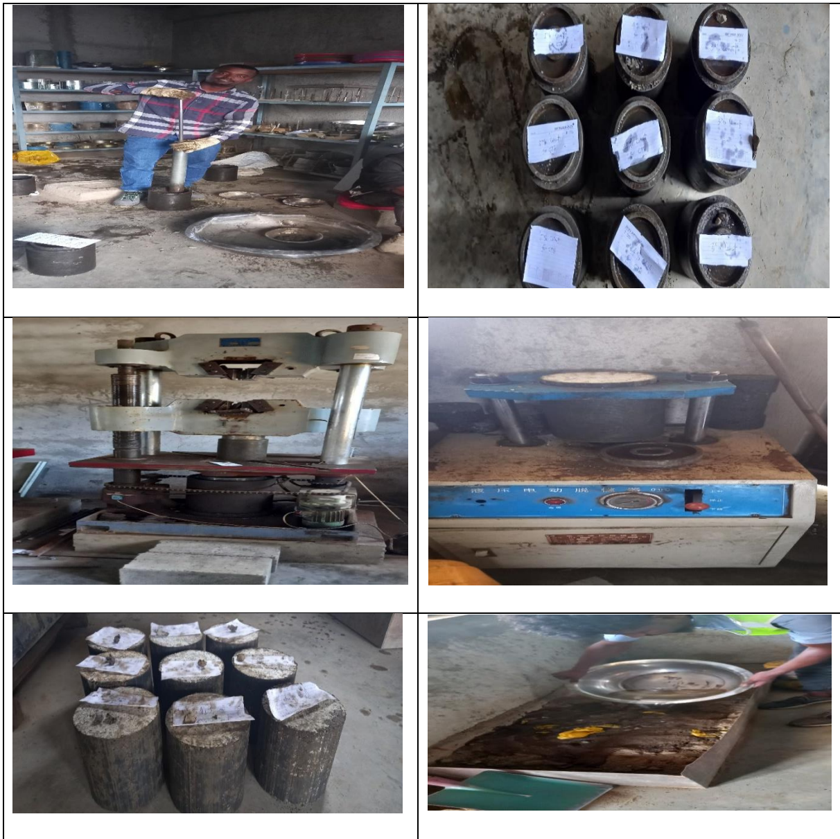
Figure 3.15 Compressive strength test procedure for compaction, demolding and curing of CTB
