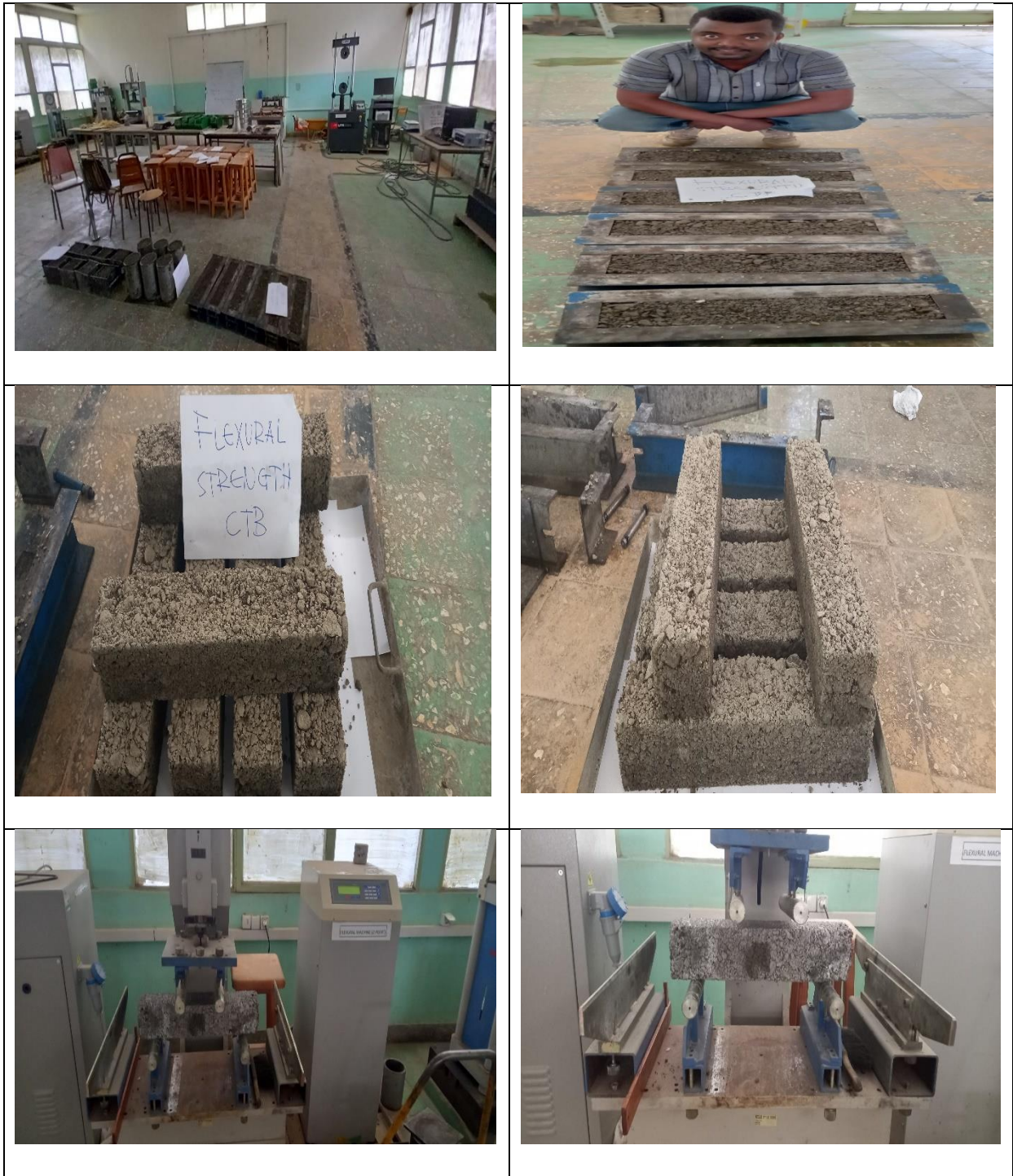
Figure 3.18 Flexural Strength (Modulus of Rupture) test procedure for CTB
