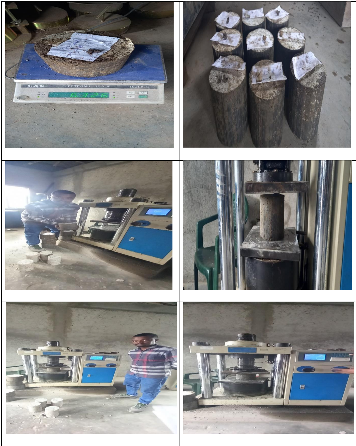
Figure 3.16 Unconfined Compressive strength test procedure for CTB
