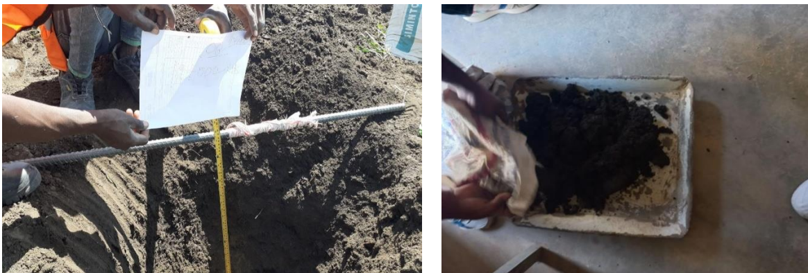
Figure 3.7 Sampling of Subgrade Soil
