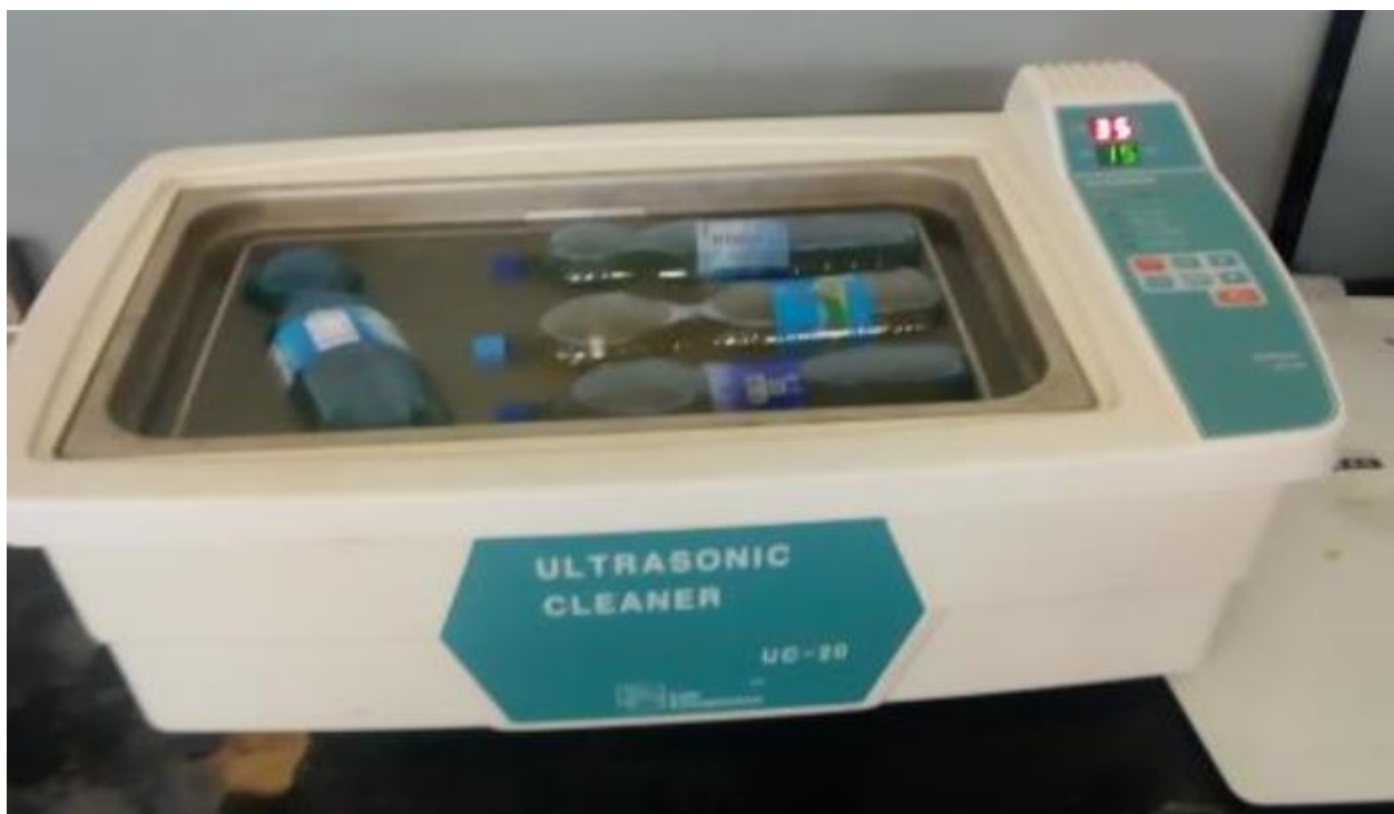
Figure 3.4 blending process utilizing the Ultrasonicator
