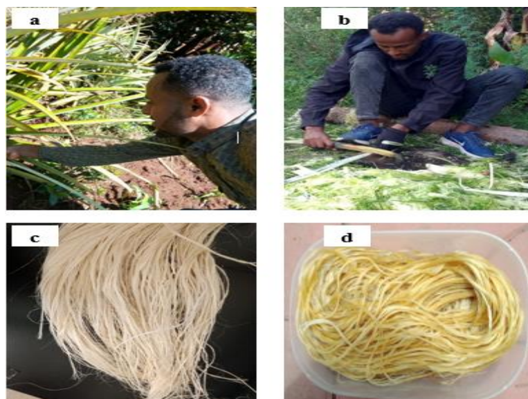
Figure 3. 1 Pineapple leaf fiber (a) harvesting plant (b) extraction process ( c) extracted fiber (d) treated fiber
