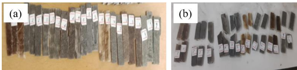
Figure 3. 21 Specimens for impact strength test (a) before test (b) after test
