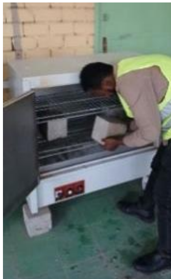
Figure 3. 17 Water absorption test
