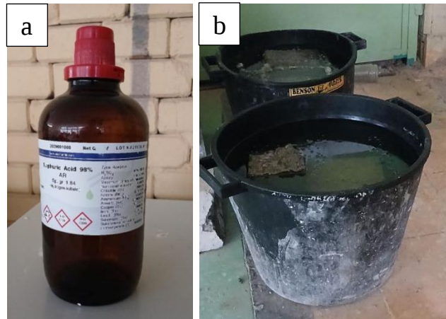
Figure 3. 16 a. Sulfuric acid b. acid attack resistance test of concrete
