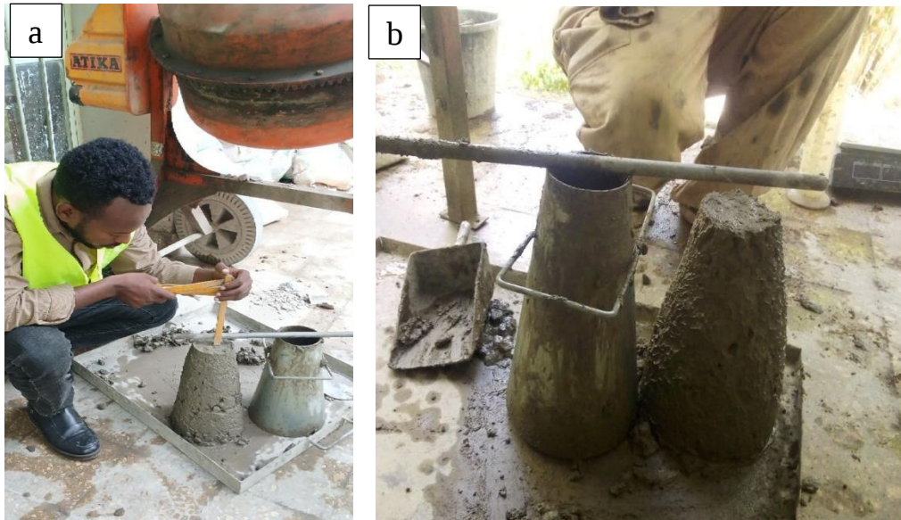
Figure 3.13 slump test of concrete a. without additive and b. with additive
