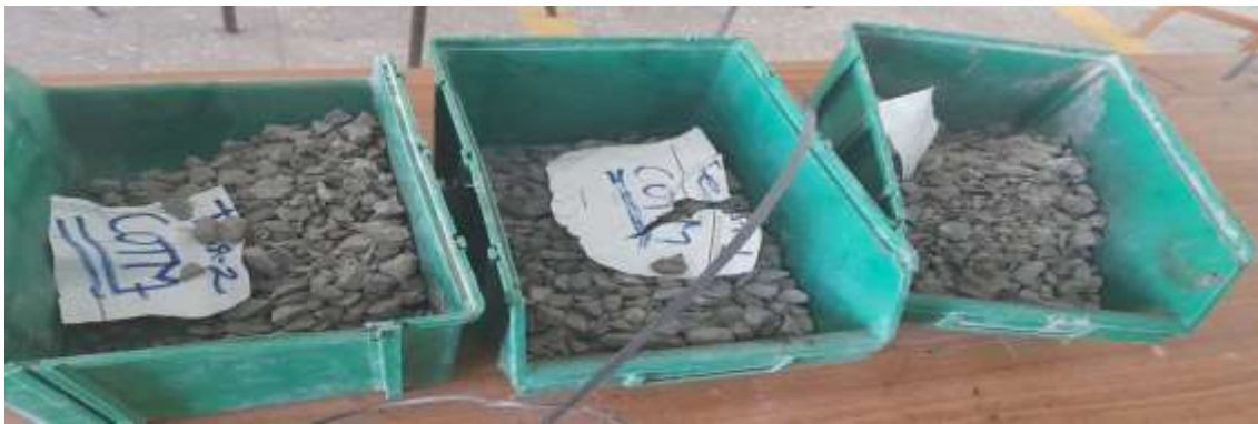
Fig 3.16 Aggregate sample that are taken for flakiness and elongation index test
