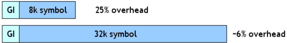
Figure 3.9: Guard interval overhead reduction with larger FFT size
