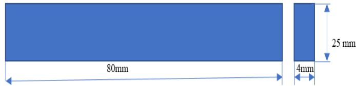
Fig. 3.21. Compression test specimen dimension
