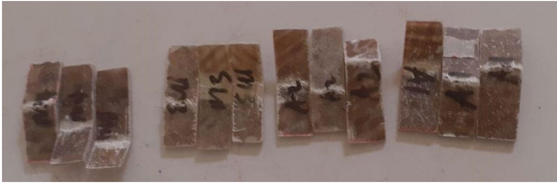
Fig. 4.18. Composite sample tested for compressive strength
