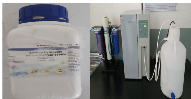
Fig. 3.13. NaOH and water distiller setup respectively
