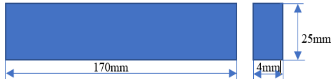
Fig. 3.22. Flexural test specimen dimension
