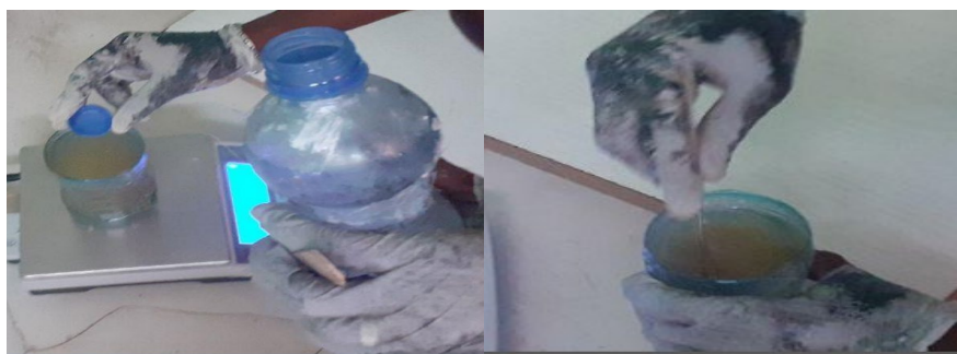
Fig. 3.2 (a). Mixing the resin and catalyst (b) Stir the mixture of resin and catalyst
