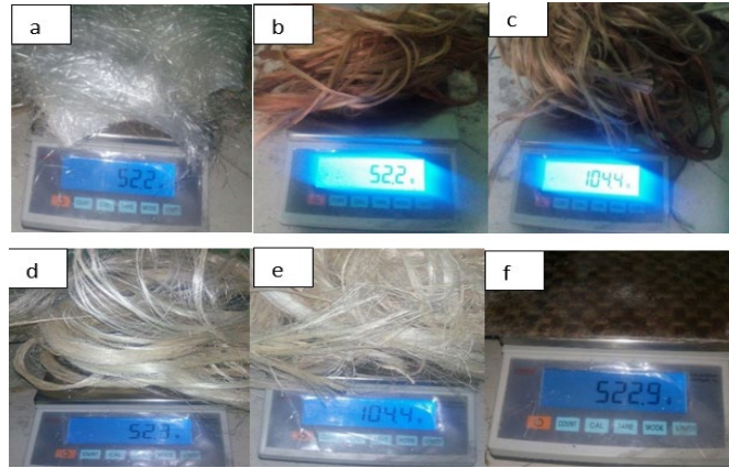
Fig. 3.11 Wight of measured fiber and composite (a)weight of glass fiber (b&c) weight of jute fiber (d & e) weight of false banana fiber (f) weight of finally made composite
