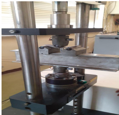
Fig. 3.26. The specimen under flexural testing
