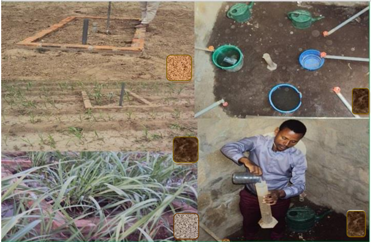
Figure 6.2: Partial view of lysimeter experiment and measuring drained water from drainage manhole
