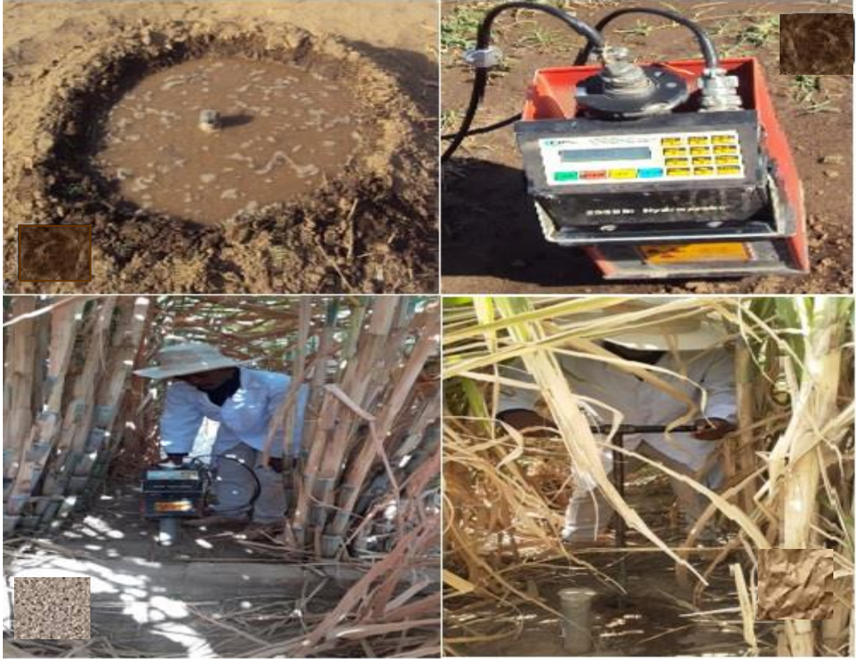
Figure 6.3: Neutron Calibration and soil moisture monitoring in the Lysimeter
