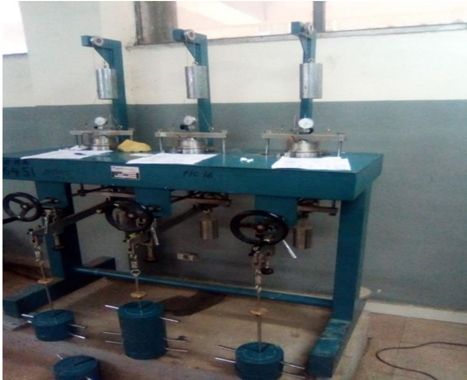
Figure 3-8: Photographic view of consolidation machine ready for data recording
