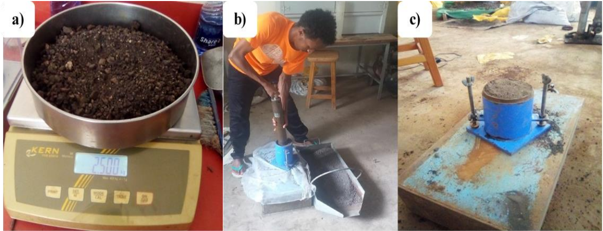
Figure 3-7: Standard compaction test (a) prepared soil sample (b) compaction operation (c) compacted sample
