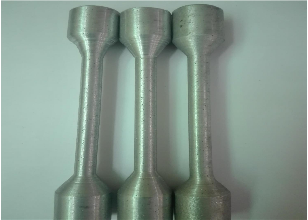
Figure 4.10. Sample specimens for tensile test
