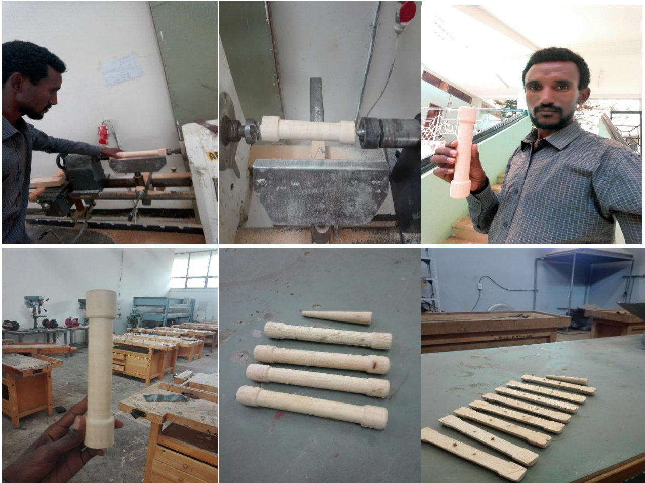
Figure 3.6. Preparation of split pattern, and sprue.
