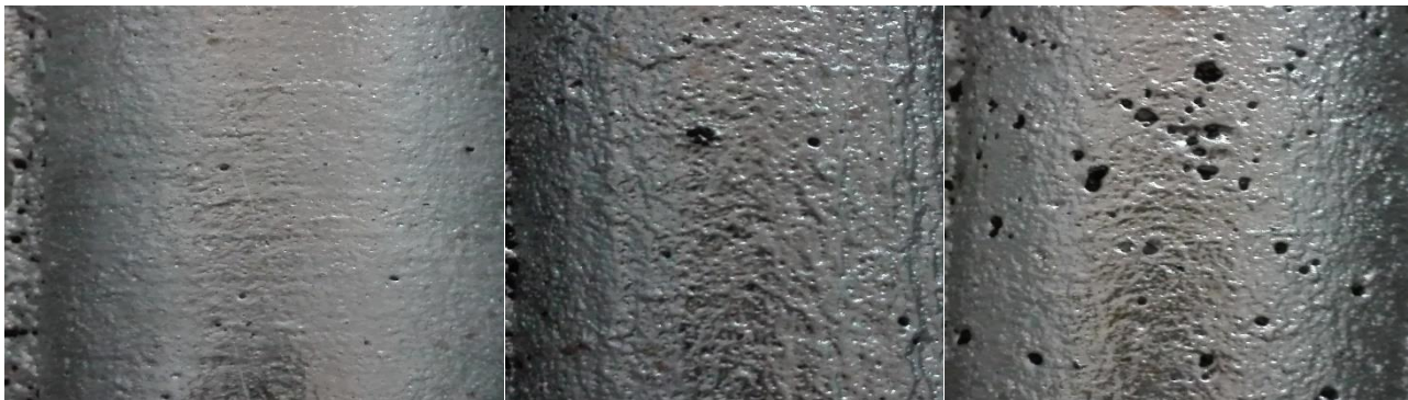
Figure 3.13. visible differences on casted samples before machining
