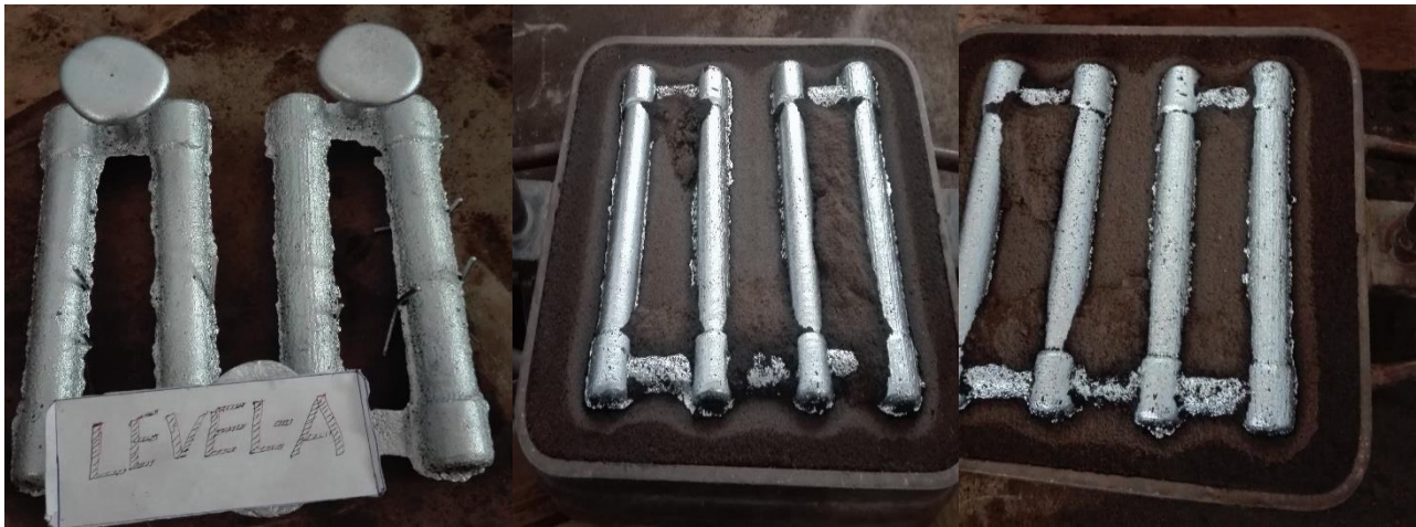
Figure 3.11. Casted samples with 3 - level of defect
