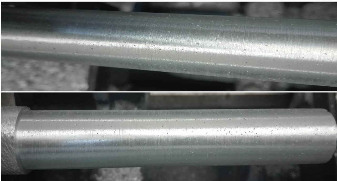
Figure 3.17. Machined surfaces on the lathe machine
