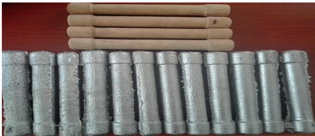
Figure 3.14. Casting samples after fettling process
