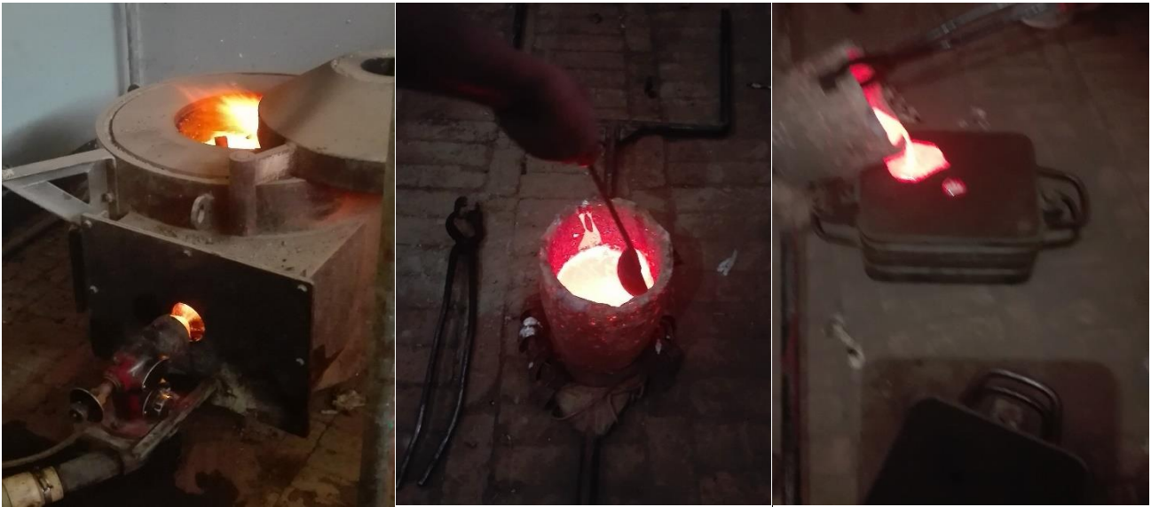
Figure 3.9. melting and pouring process
