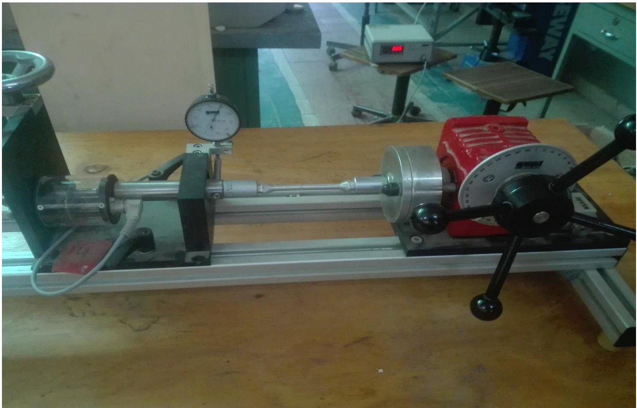
Figure 4.11. Torsion test set up
