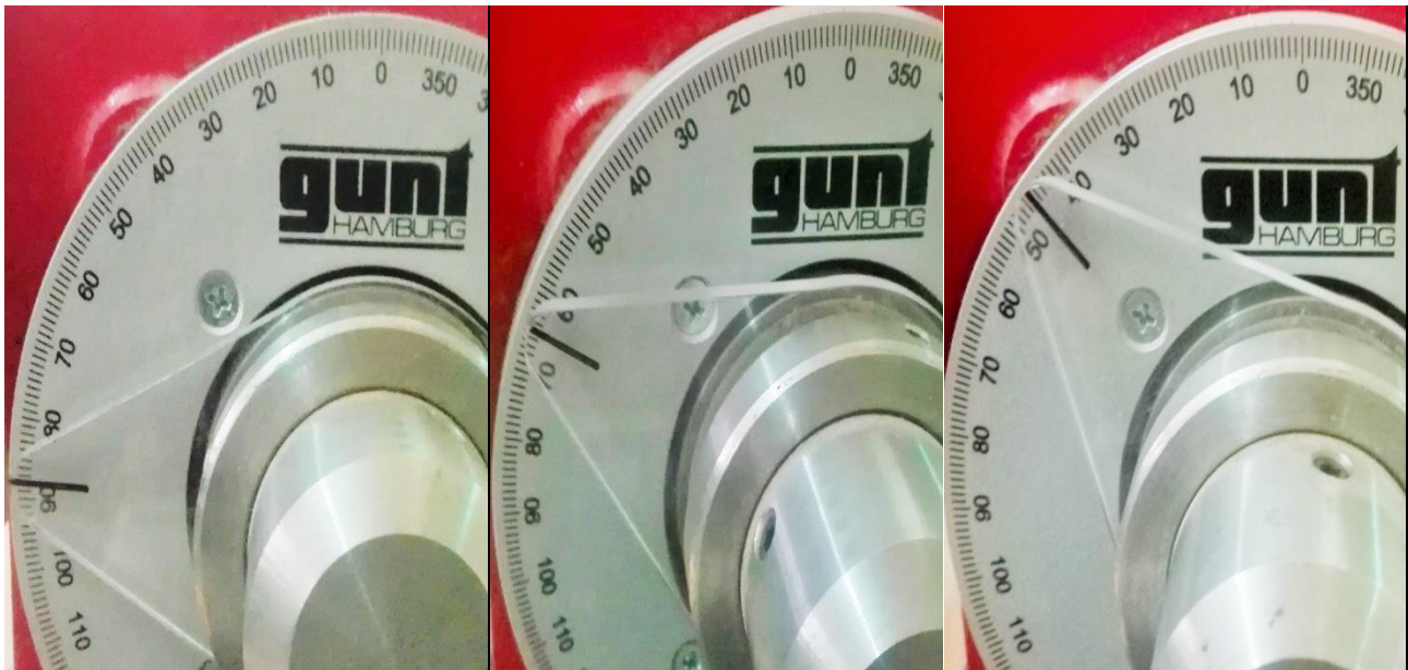
Figure 4.12. Result of the experiment from the testing machine (a) torque (b) twist angle
